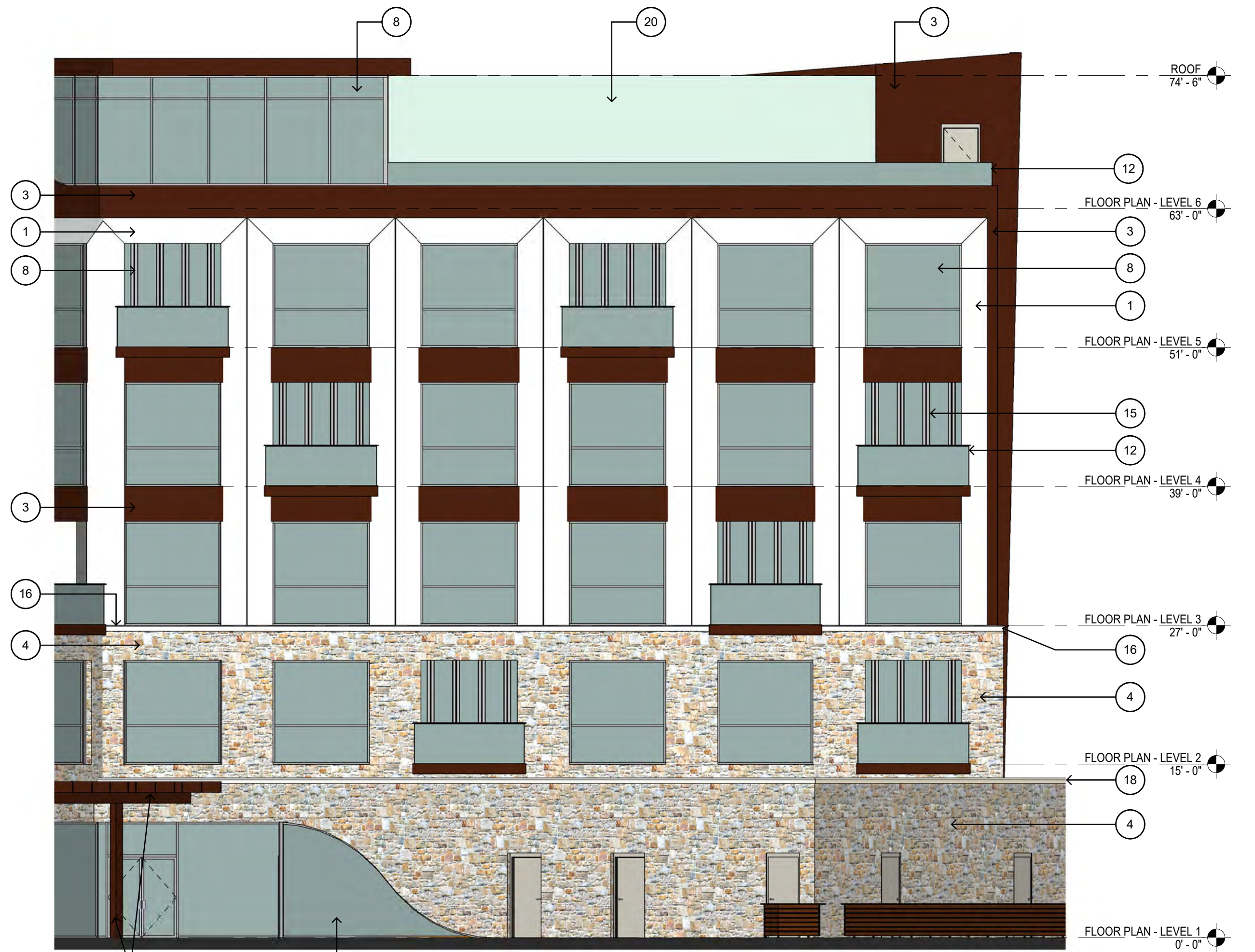
3 BUILDING 1- SOUTHWEST FACADE SCALE: 1/8" = 1'-0"
