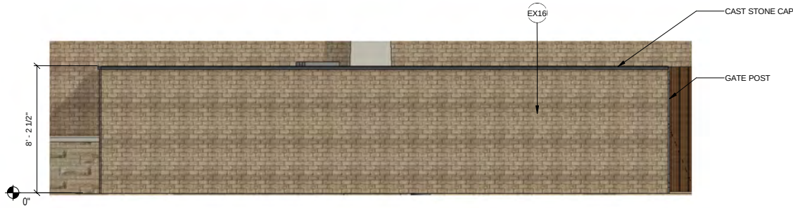
DUMPSTER ENCLOSURE EAST ELEV.
