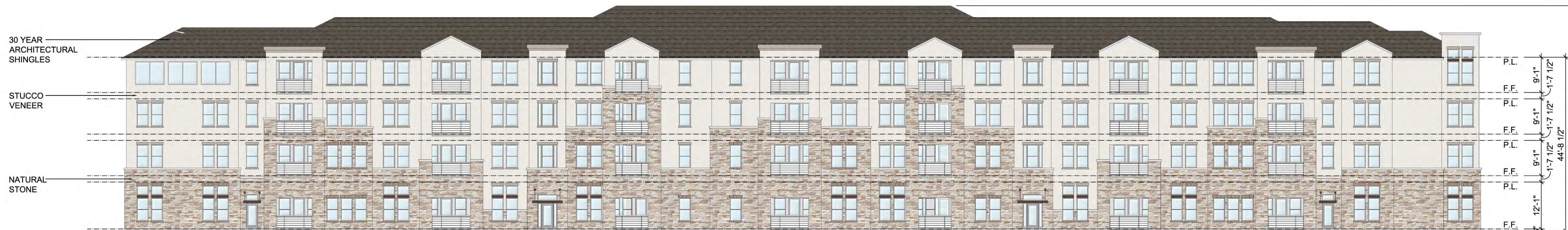
03 BUILDING TYPE 'A' NORTH ELEVATION SCALE: 1/16" = 1'-0"
