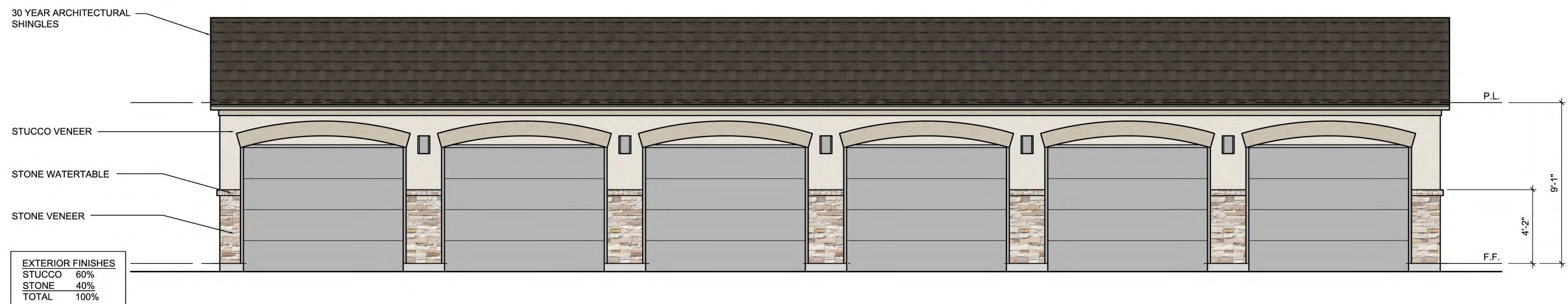
01 6-BAY GARAGE FRONT ELEVATION 1/4" = 1'-0"
