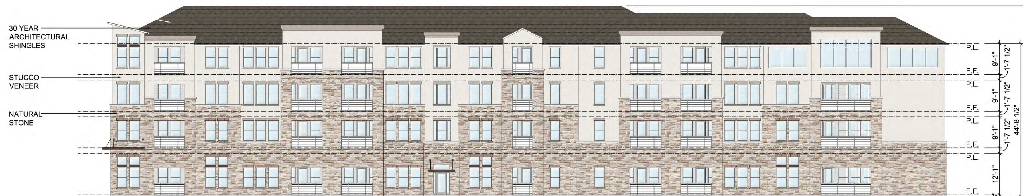
02 BUILDING TYPE 'A' EAST ELEVATION SCALE: 1/16" = 1'-0"
