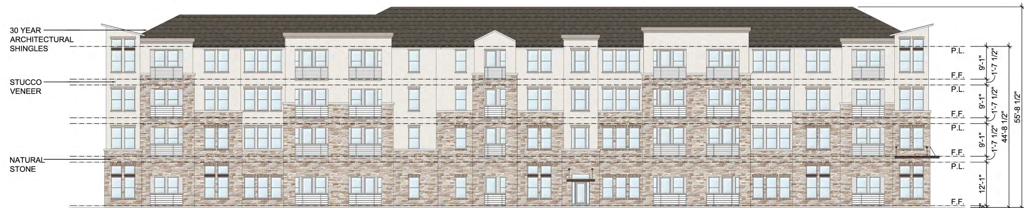
04 BUILDING TYPE 'A' WEST ELEVATION SCALE: 1/16" = 1'-0"
