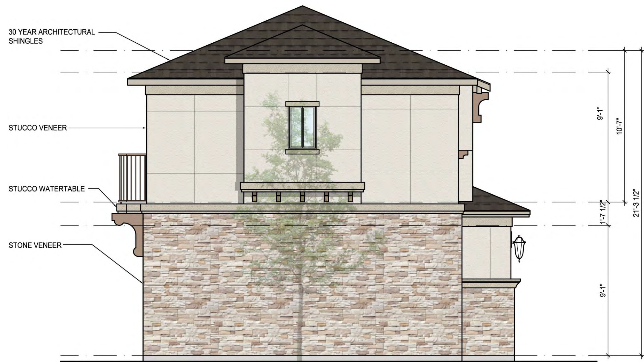
03 BUILDING 'B' - LEFT ELEVATION SCALE: 1/4" = 1'-0"
