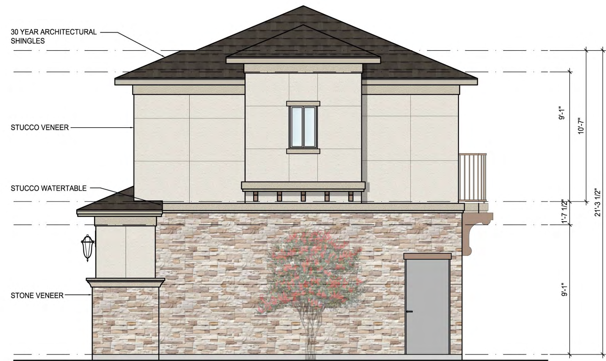
02 BUILDING 'B' - RIGHT ELEVATION SCALE: 1/4" = 1'-0"
