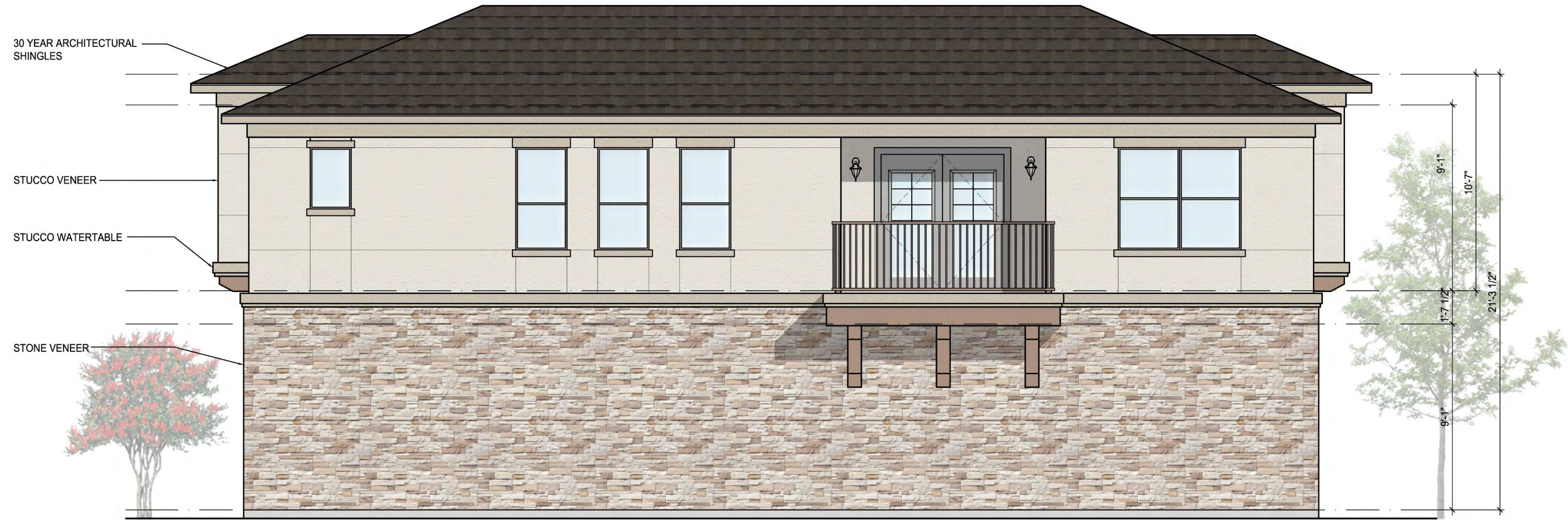
04 BUILDING 'B' - REAR ELEVATION SCALE: 1/4" = 1'-0"
