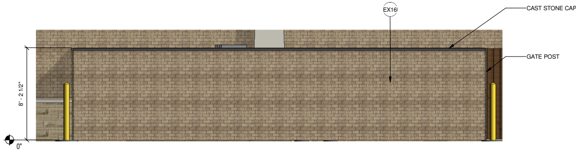
DUMPSTER ENCLOSURE EAST ELEV.
