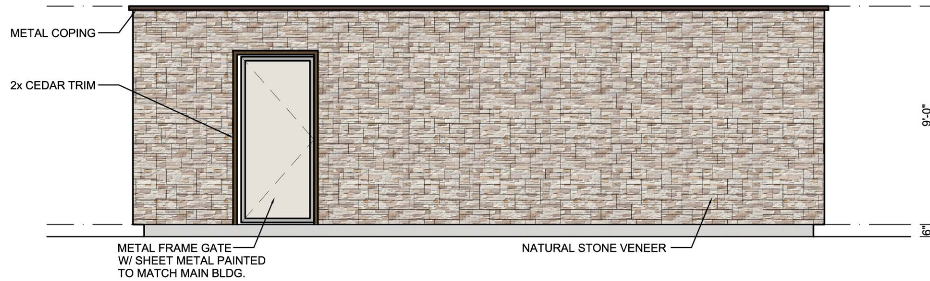
02 TRASH COMPACTOR - RIGHT ELEVATION 1/4" = 1'-0"
