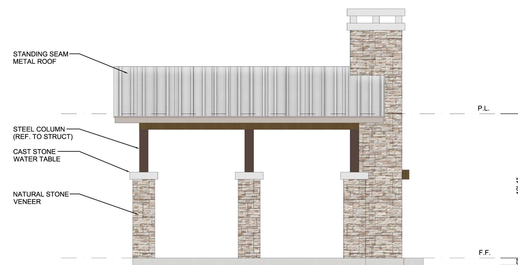
01 PAVILION - RIGHT ELEVATION 1/4" = 1'-0"
