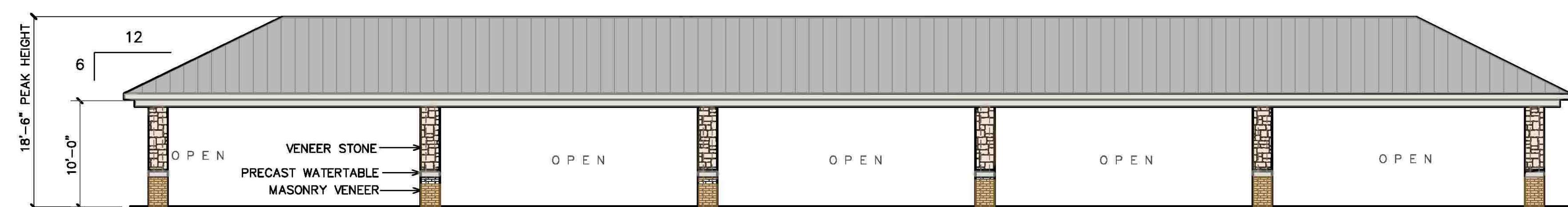
2 CA2 EAST ELEVATION - VACUUM CANOPY 1/8"=1'-0"
