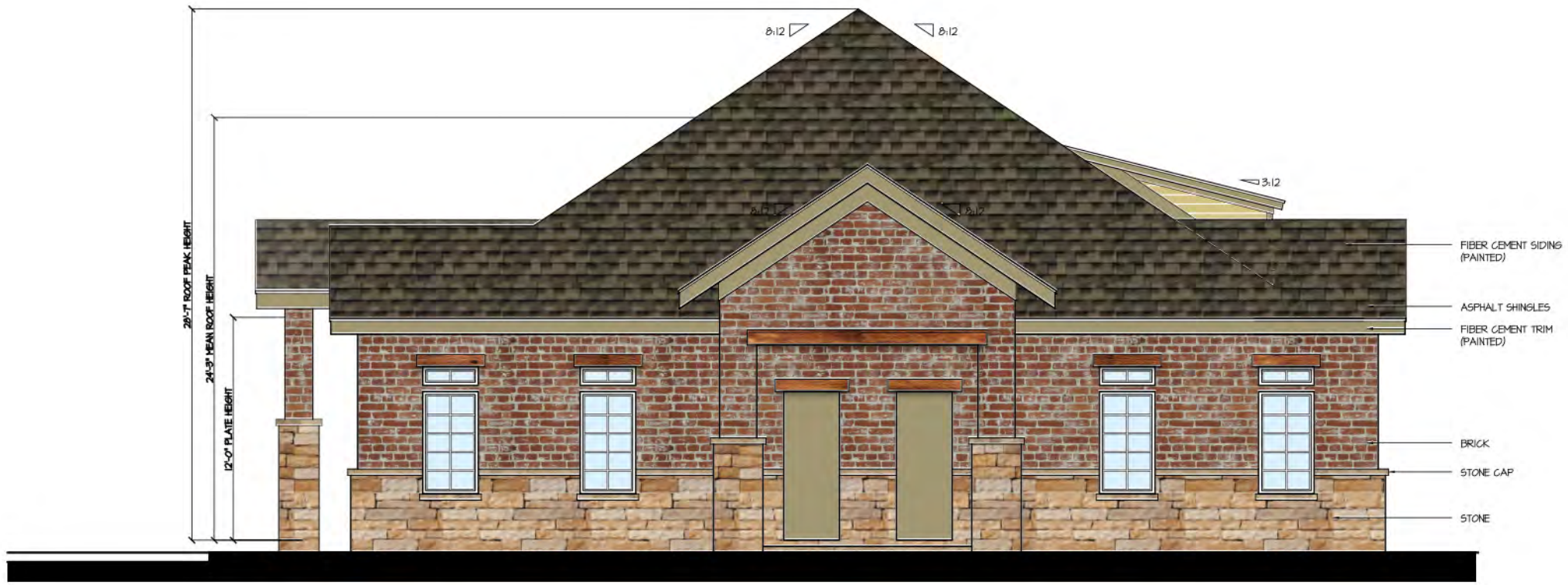
1 OFFICE BUILDING : WEST ELEVATION SCALE: 1/8" = 1'-0" (24"X36")
