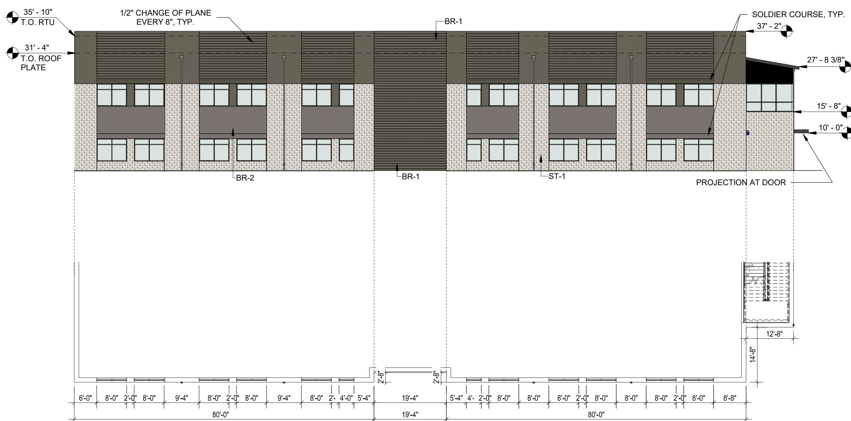
04 EXTERIOR ELEVATION- CR BLOCK SOUTH 1/16" = 1'-0"
