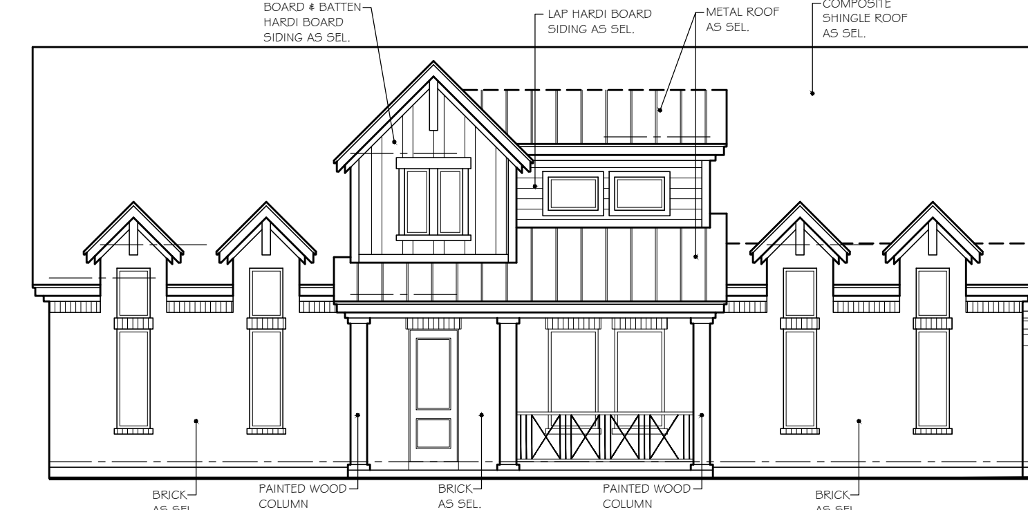
FRONT (SOUTH) ELEVATION (TYPE M - A) 1/8" = 1' - 0" scale
