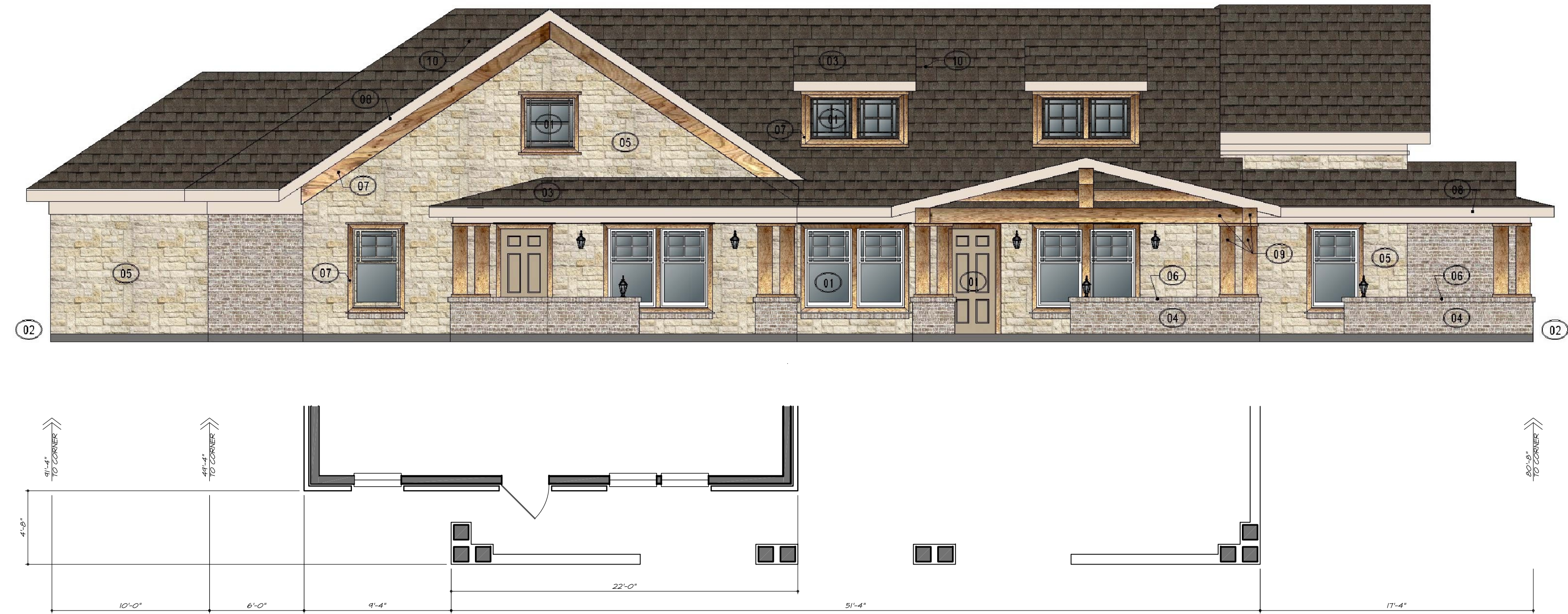
01 EXTERIOR ELEVATION - EAST SIDE FACING MORRIS SCALE: 1/4"=1'-0"
