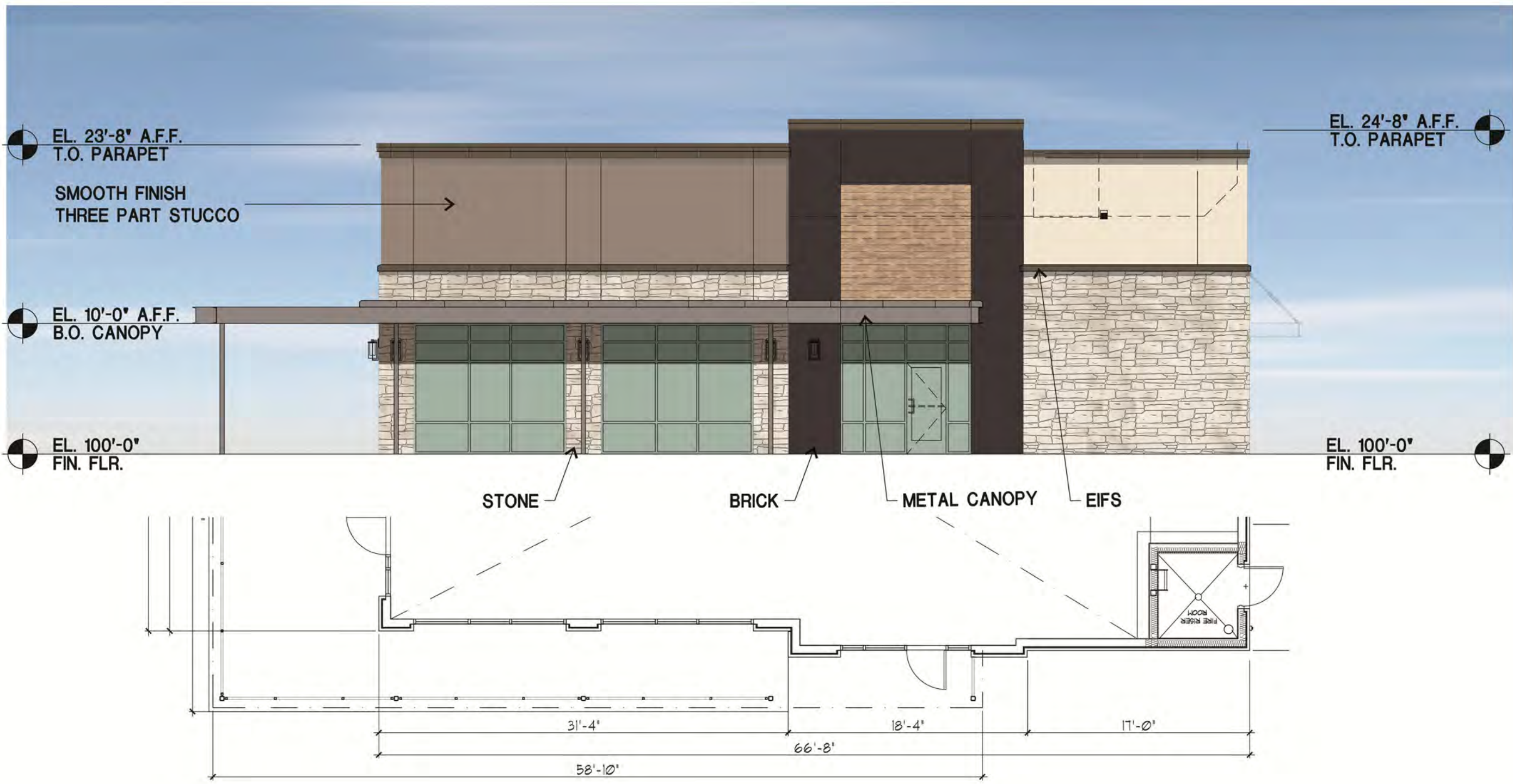
02 SIDE (NORTH) ELEVATION
