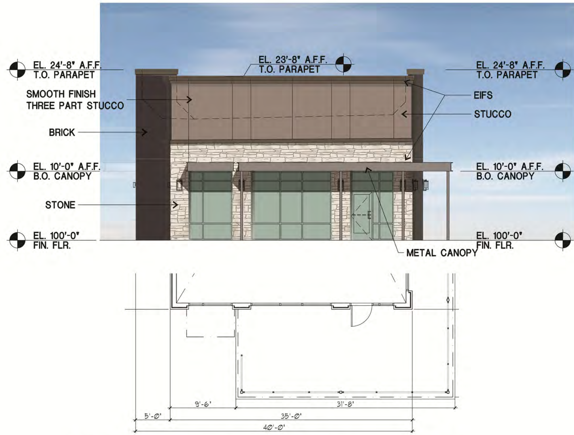
01 FRONT (EAST) ELEVATION
