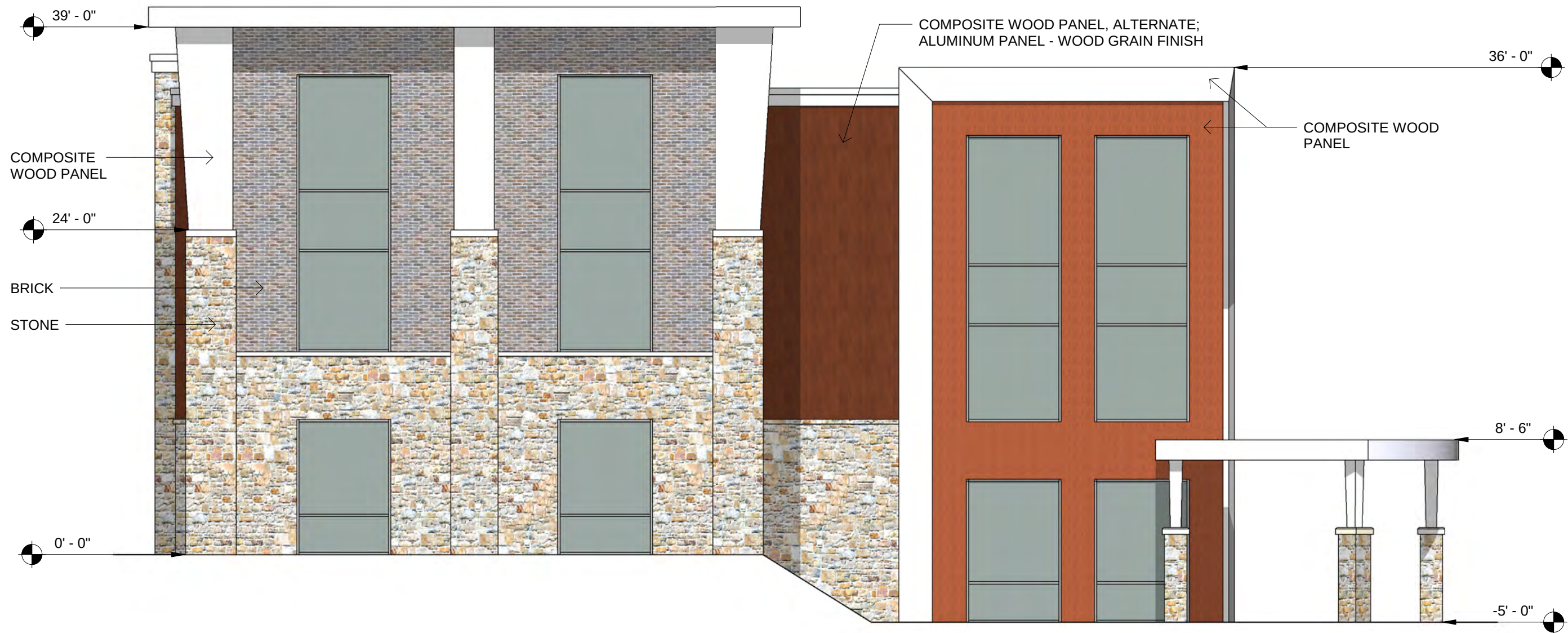
② BUILDING 6 - ELEVATION - NORTH 1/8" = 1'-0"
