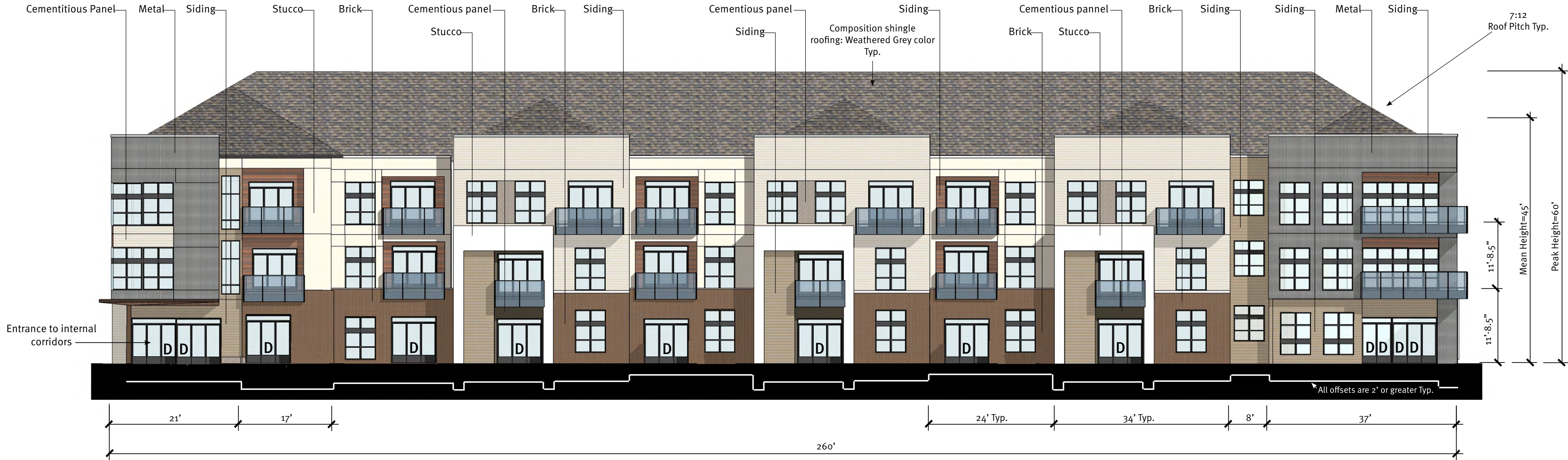
01 Typical Multi Family Building - Front Elevation (West)
