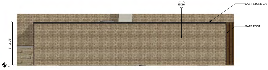
DUMPSTER ENCLOSURE EAST ELEV.
