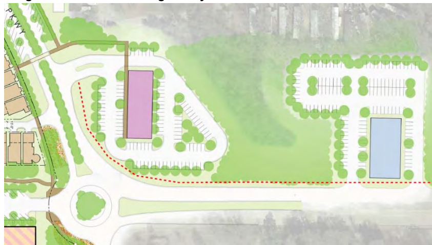
Figure 10: Lakeside Village Pkwy sidewalk extension
