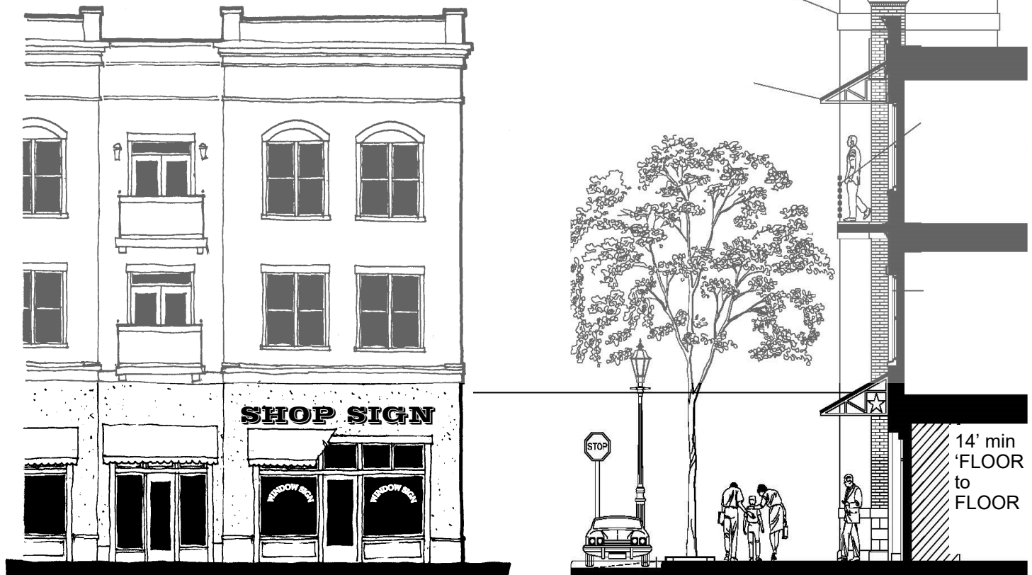
Figure 7.2: Ground floor built to commercial standards
