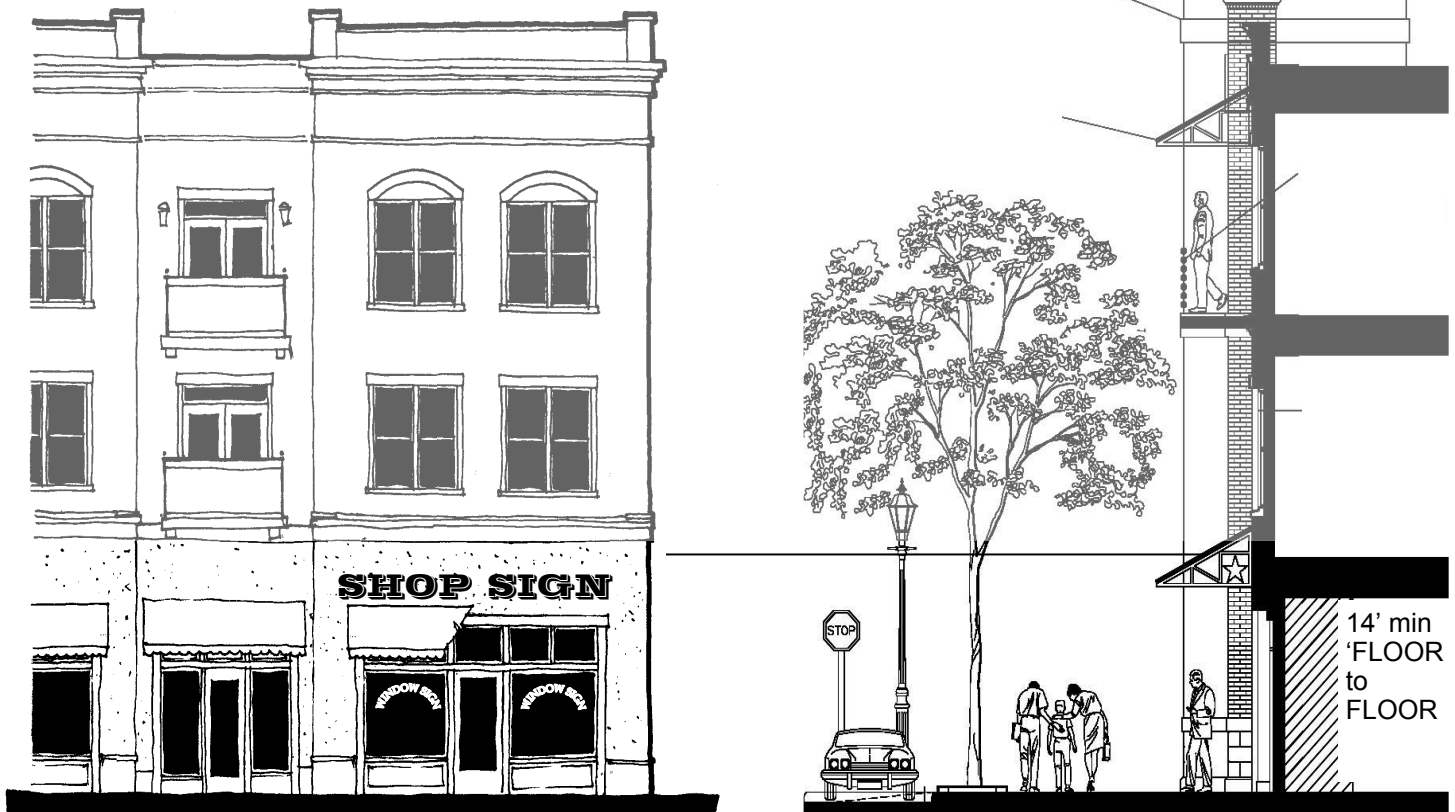
Figure 7.2: Ground floor built to commercial standards
