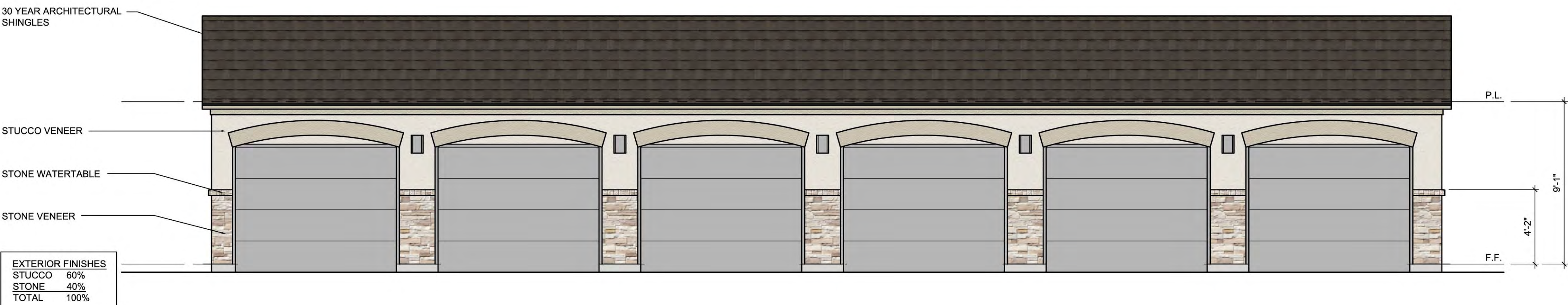
01 6-BAY GARAGE FRONT ELEVATION 1/4" = 1'-0"
