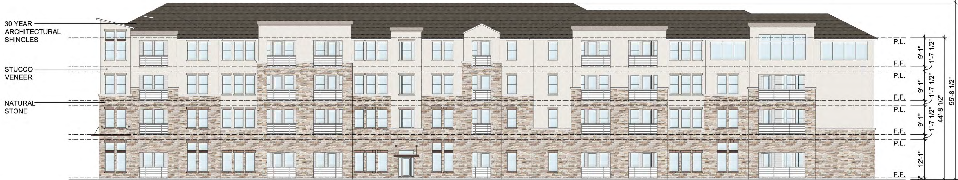
02 BUILDING TYPE 'A' EAST ELEVATION SCALE: 1/16" = 1'-0"
