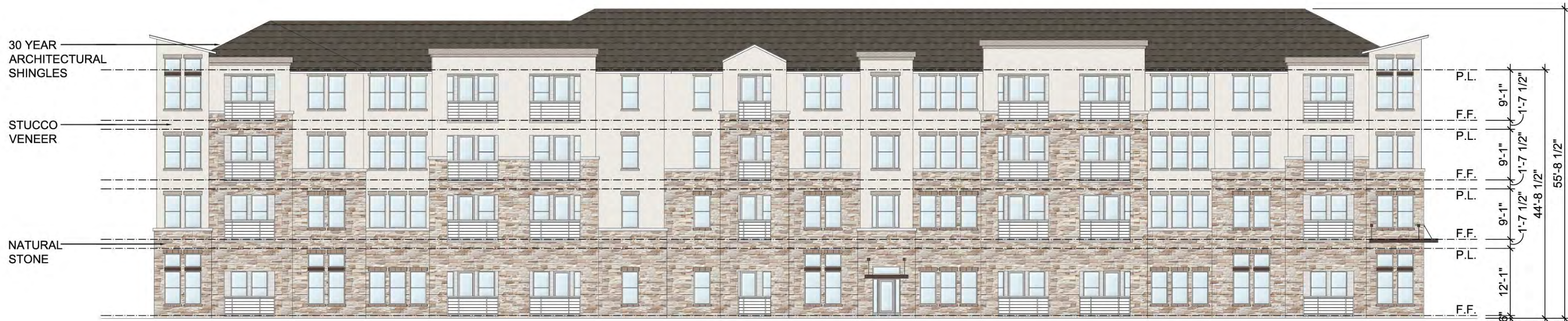
04 BUILDING TYPE 'A' WEST ELEVATION SCALE: 1/16" = 1'-0"
