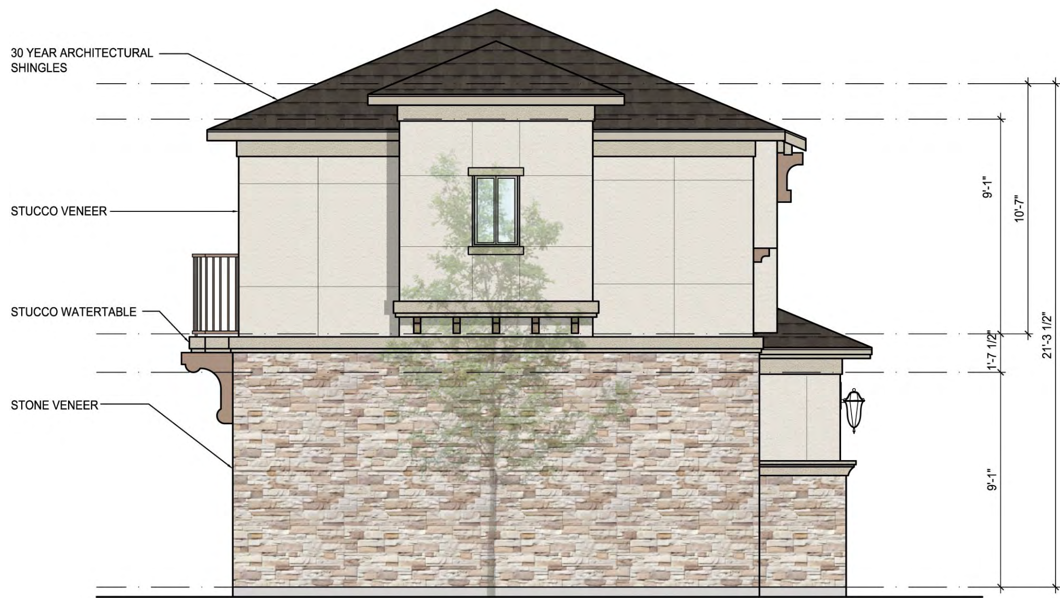
03 BUILDING 'B' - LEFT ELEVATION SCALE: 1/4" = 1'-0"
