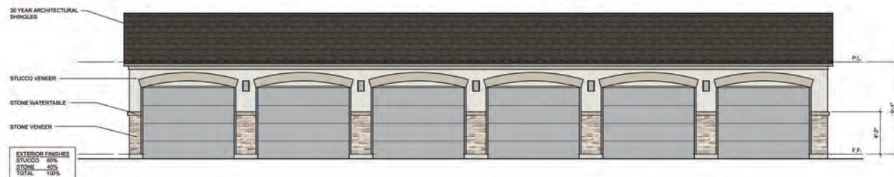
01 6-BAY GARAGE FRONT ELEVATION 1/4" = 1'-0"
