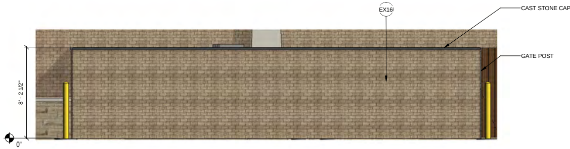
DUMPSTER ENCLOSURE EAST ELEV.
