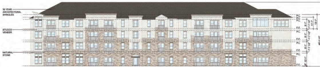
02 BUILDING TYPE 'A' WEST ELEVATION SCALE: 1/16" = 1'-0"
