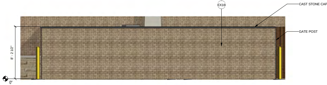
DUMPSTER ENCLOSURE EAST ELEV.
