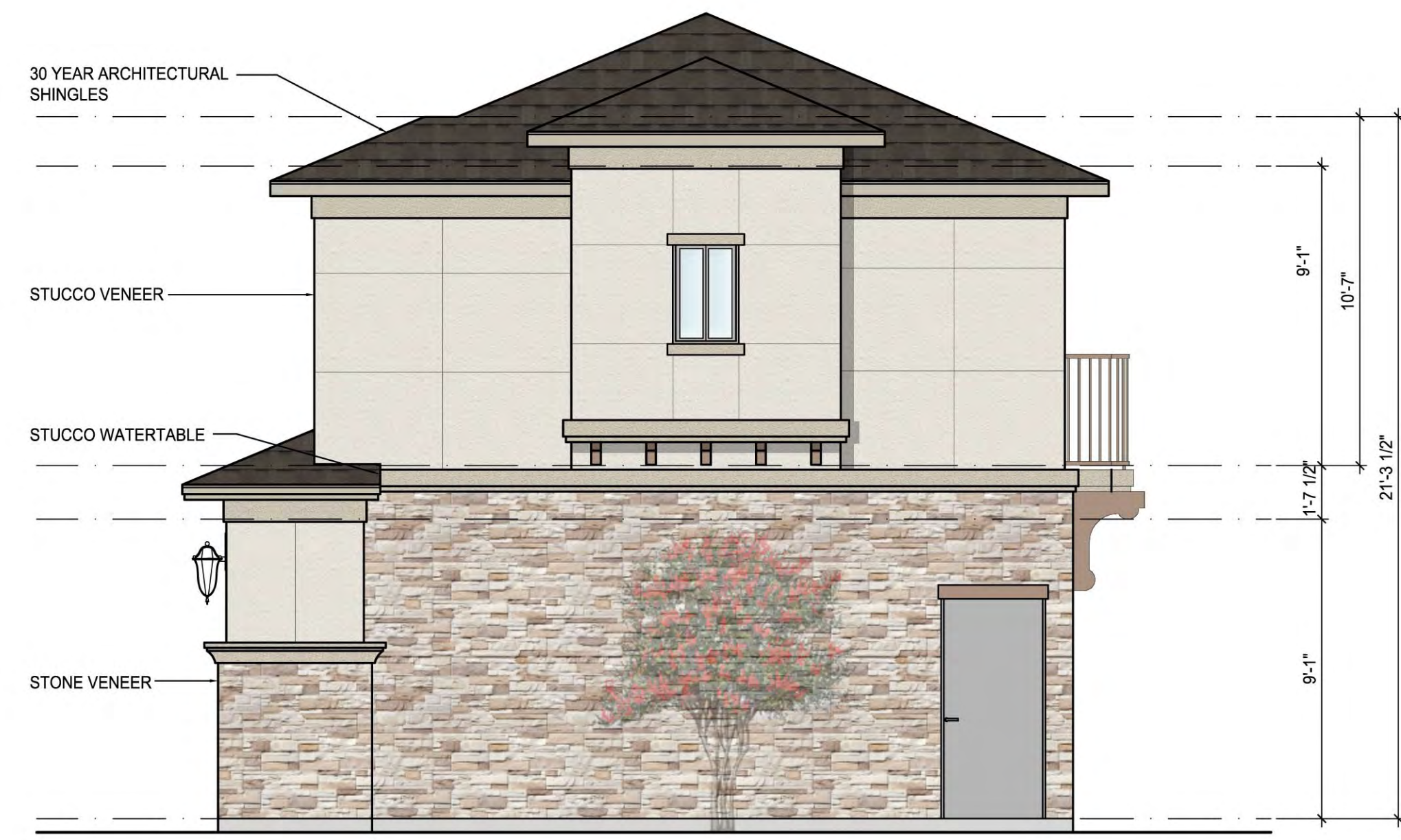
02 BUILDING 'B' - RIGHT ELEVATION SCALE: 1/4" = 1'-0"
