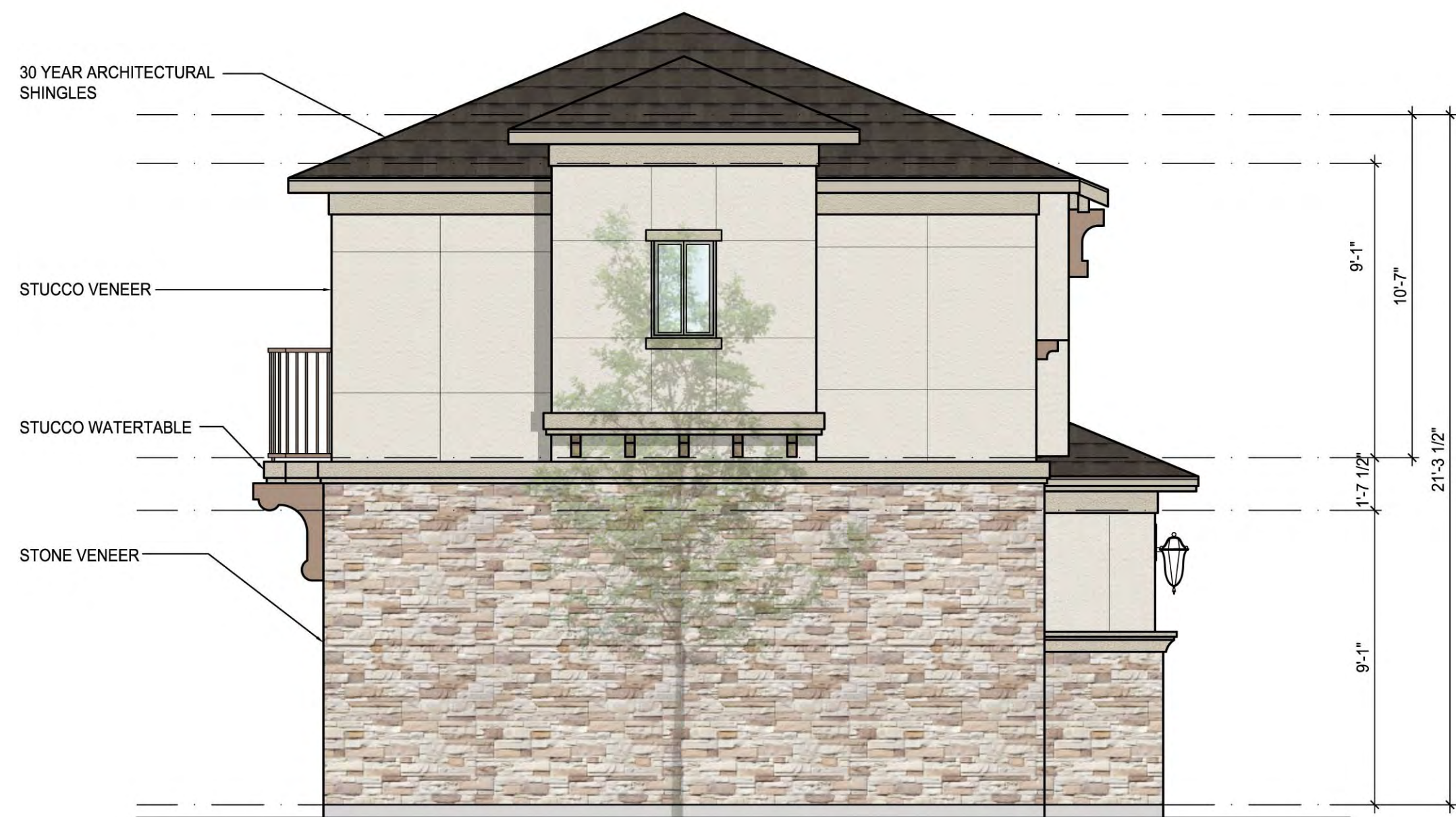
03 BUILDING 'B' - LEFT ELEVATION SCALE: 1/4" = 1'-0"
