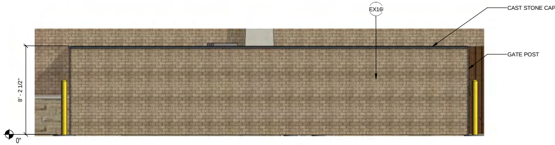
DUMPSTER ENCLOSURE EAST ELEV.
