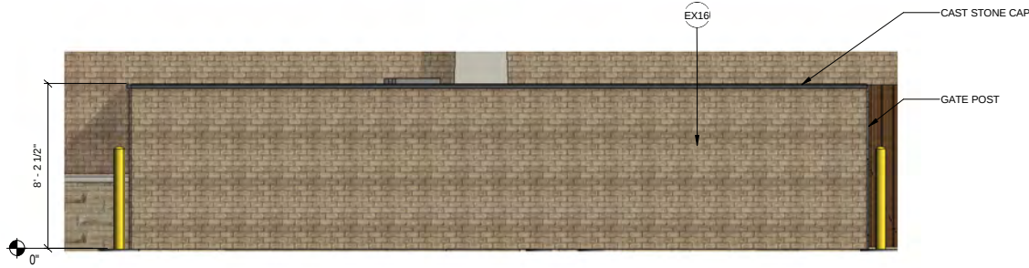
DUMPSTER ENCLOSURE EAST ELEV.
