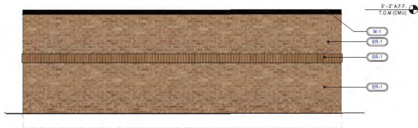
2 DUMPSTER ENCLOSURE REAR ELEVATION 3/8" = 1'-0"
