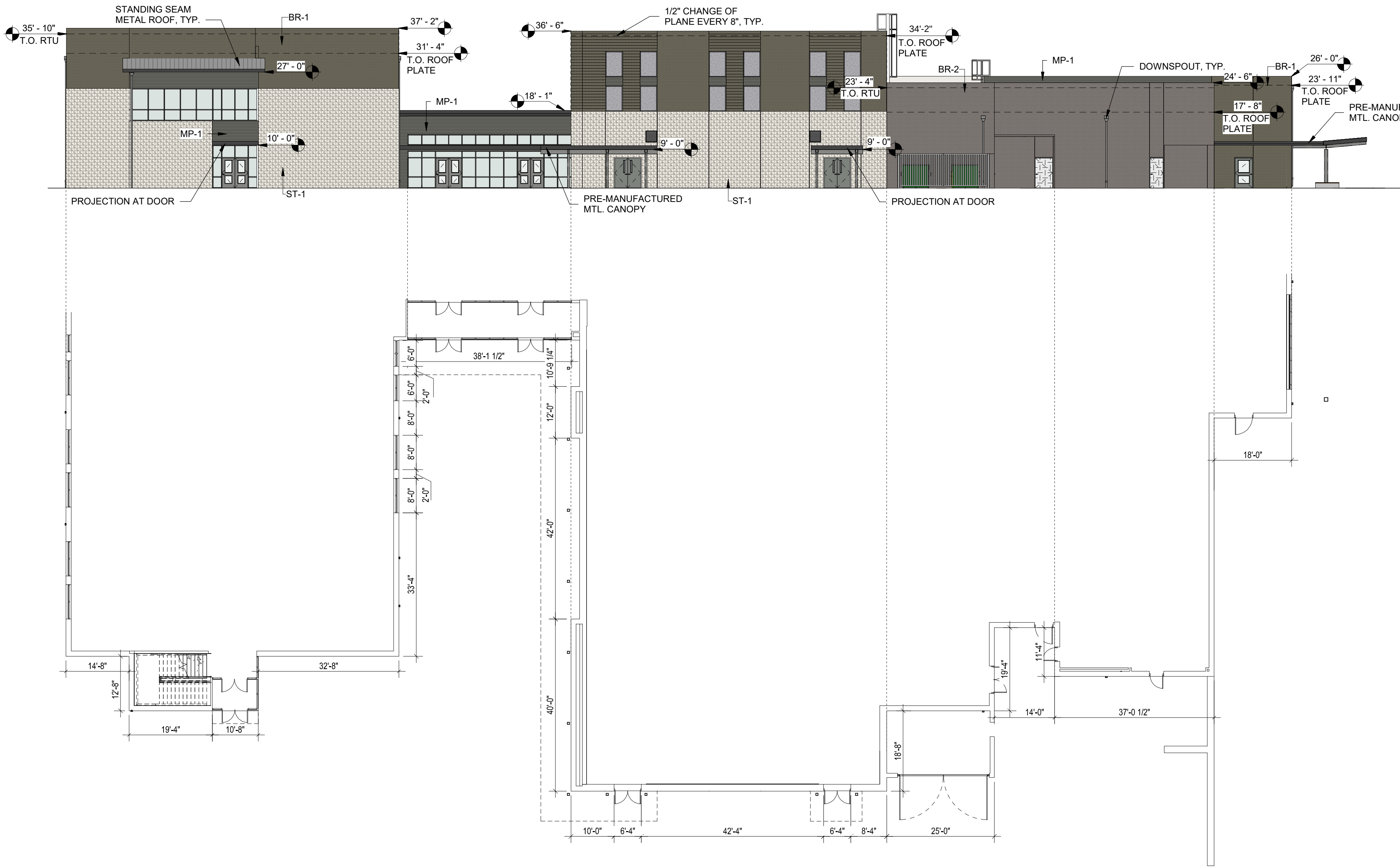
01 WEST - OVERALL ELEVATION 1/16" = 1'-0"
