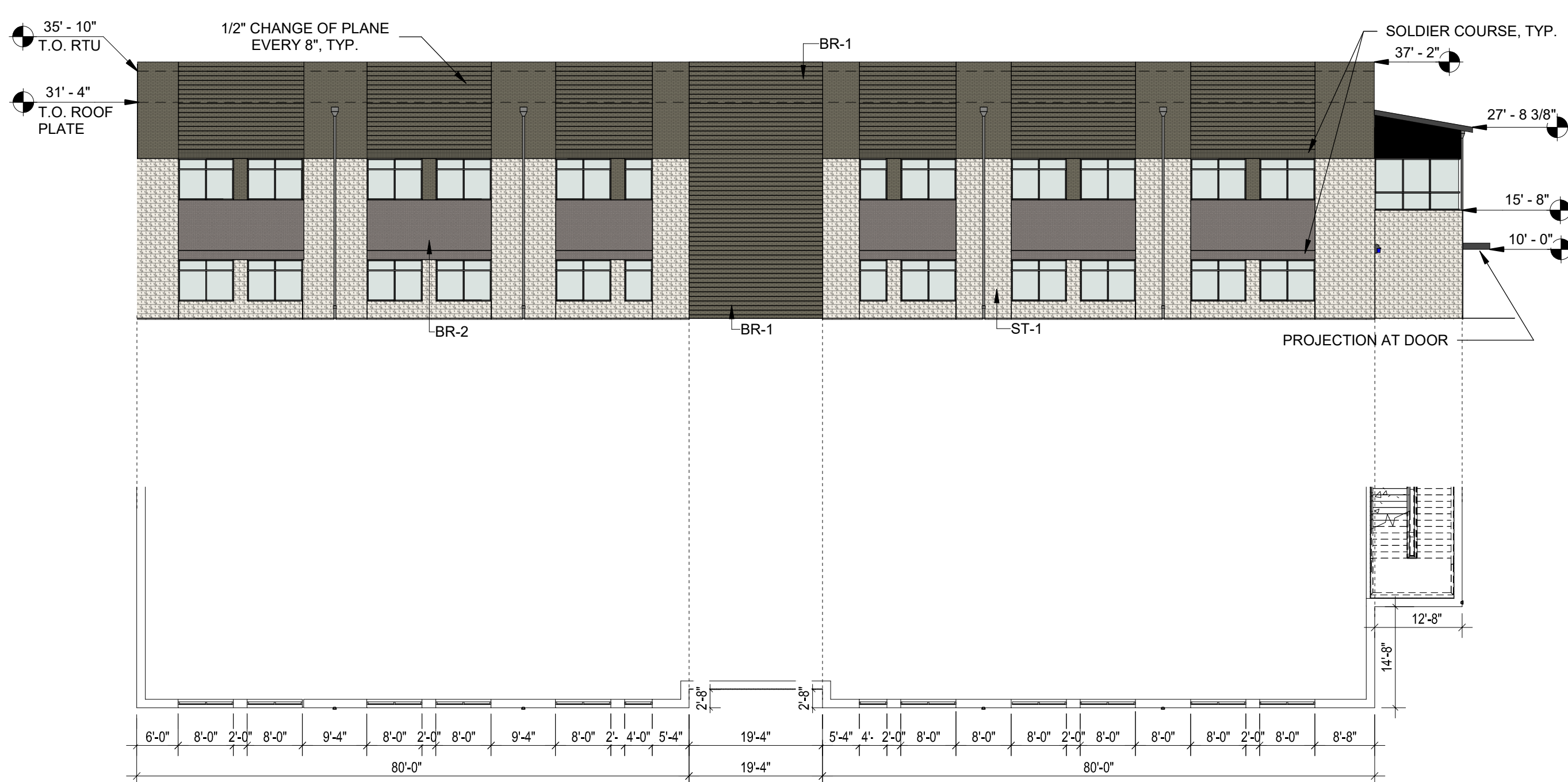
04 EXTERIOR ELEVATION- CR BLOCK SOUTH 1/16" = 1'-0"
