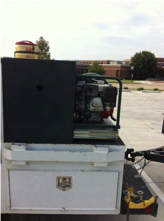
Dakota Bodies Inc Line Body 144 inches long x 63 inches high x 96 inches wide
