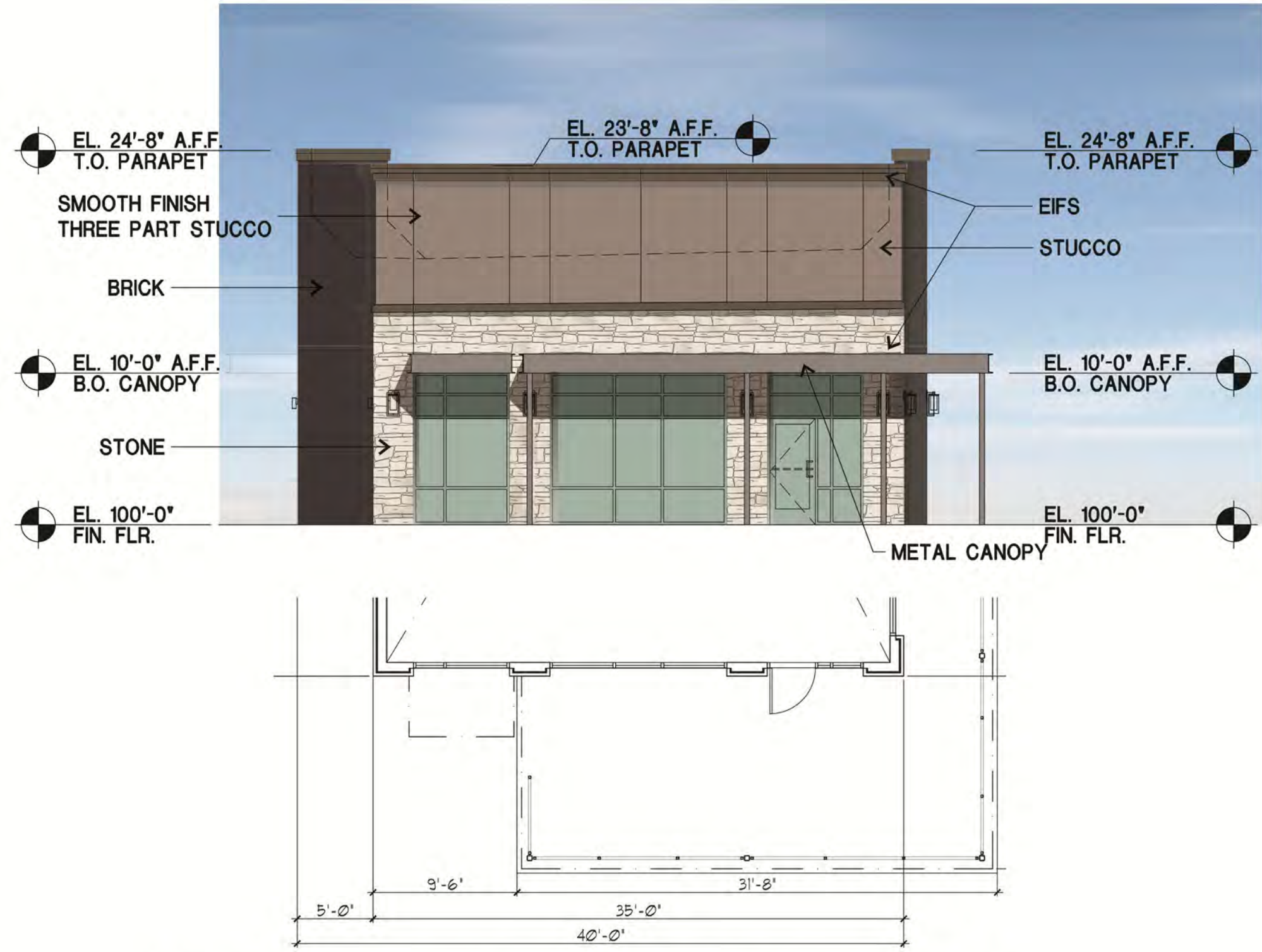
01 FRONT (EAST) ELEVATION
