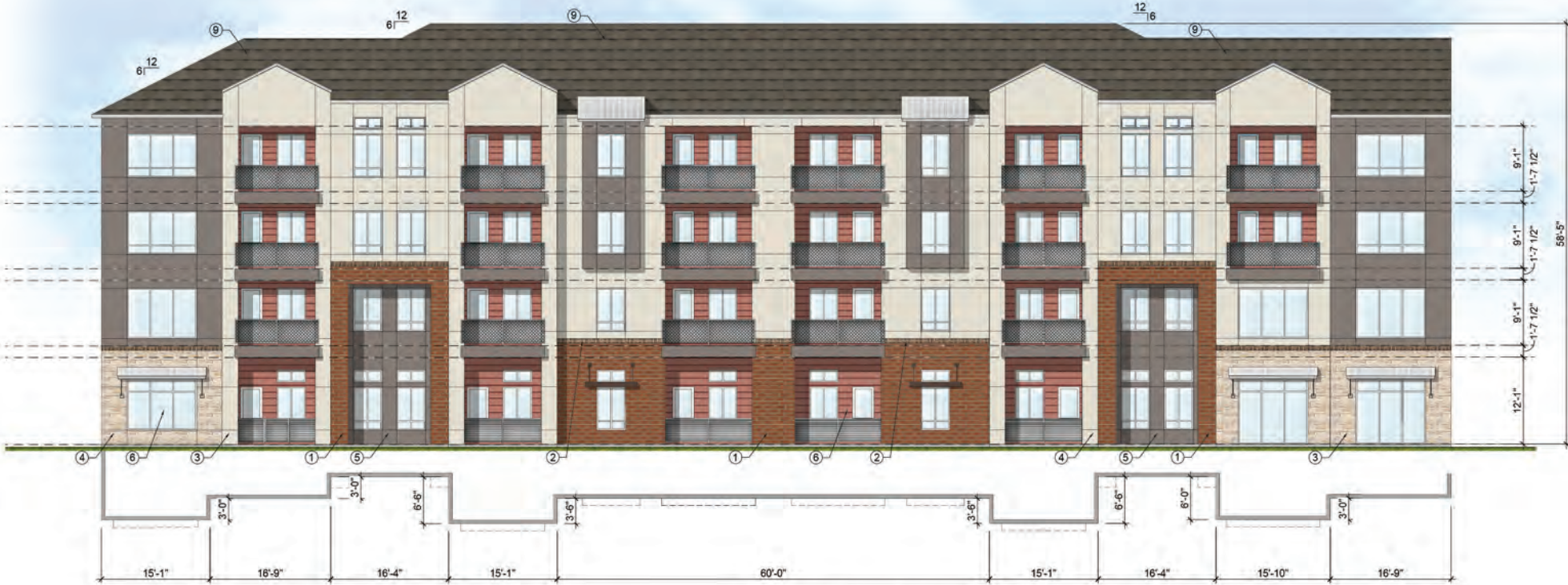
MULTIFAMILY SOUTHWEST ELEVATION
