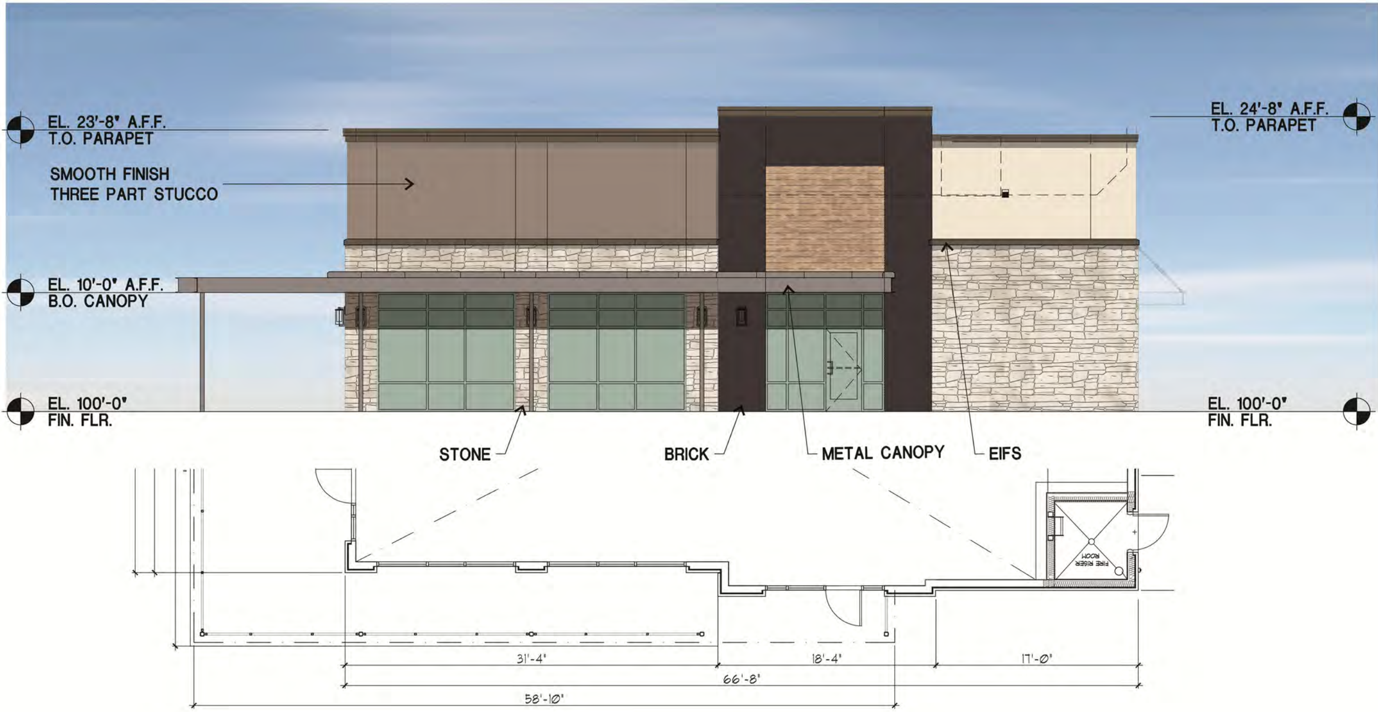
02 SIDE (NORTH) ELEVATION
