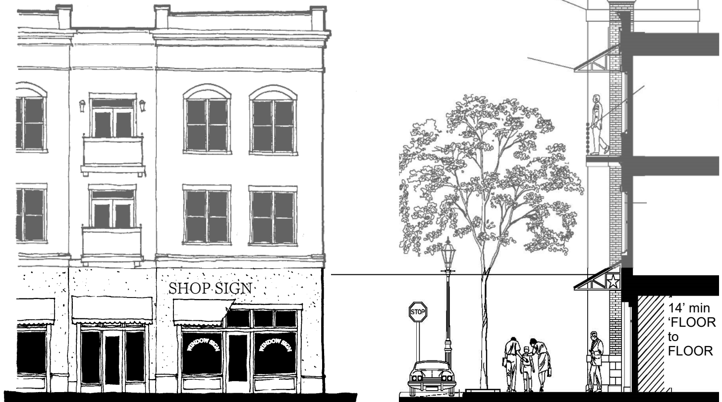
Figure 7.2: Ground floor built to commercial standards
