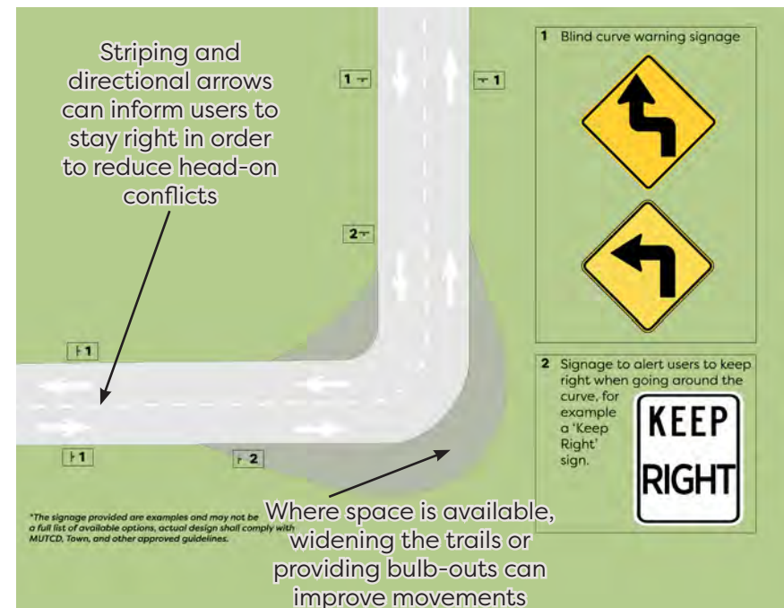
FIGURE 5.3: TYPICAL BLIND CURVE DESIGN
