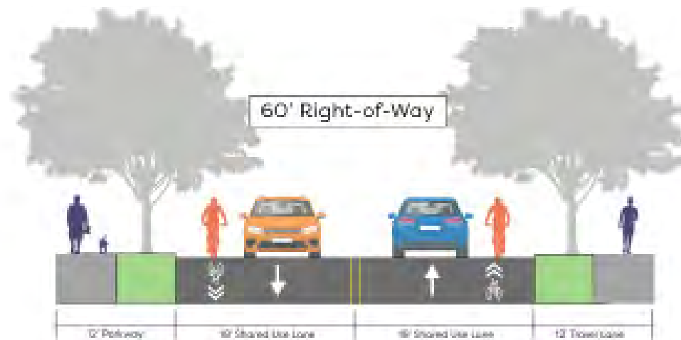
FIGURE 5.22: URBAN COLLECTOR PROPOSED CROSS-SECTION
