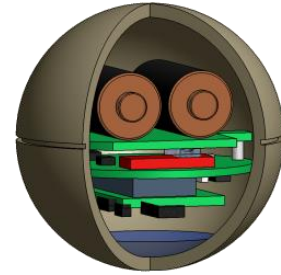
Aluminum core containing instrumentation and battery power.
