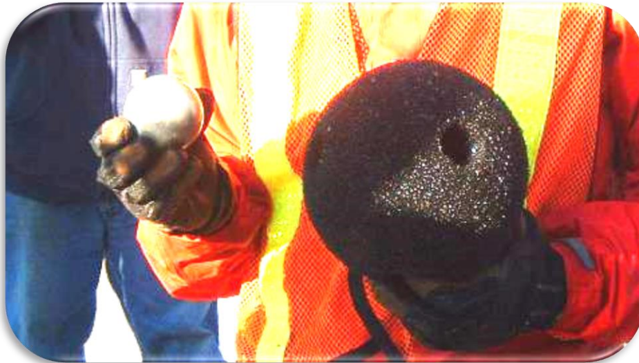
Aluminum core and outer foam protective ball.
