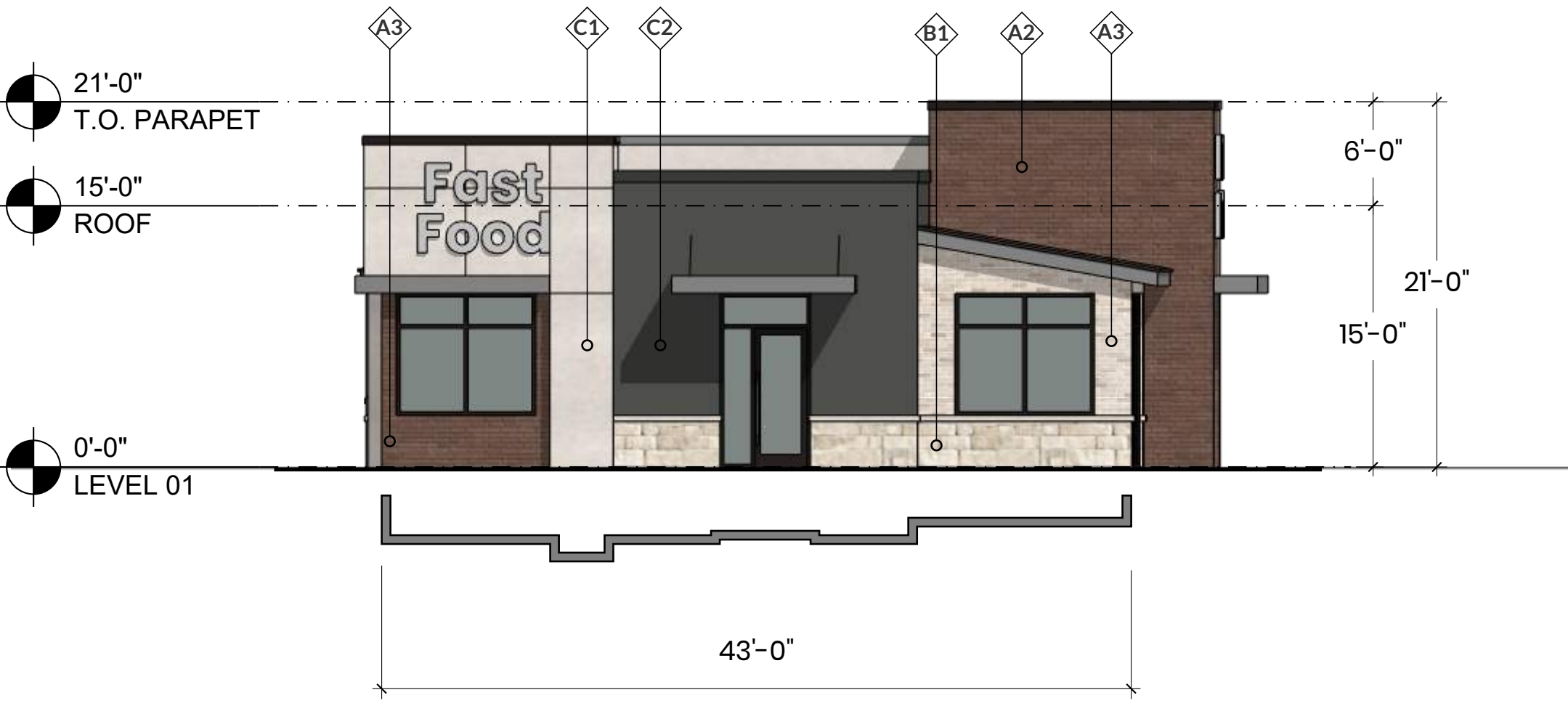
3 LEFT ELEVATION - FAST FOOD USER SCALE: 1/8" = 1'-0"
