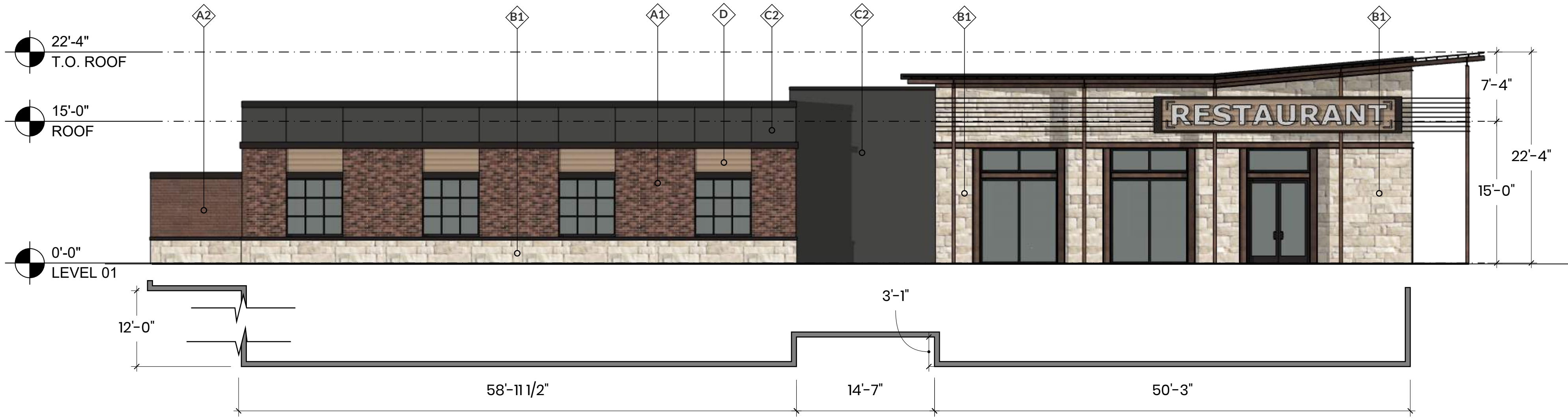
4 FRONT ELEVATION - SIT-DOWN RESTARAUNT SCALE: 1/8" = 1'-0"
