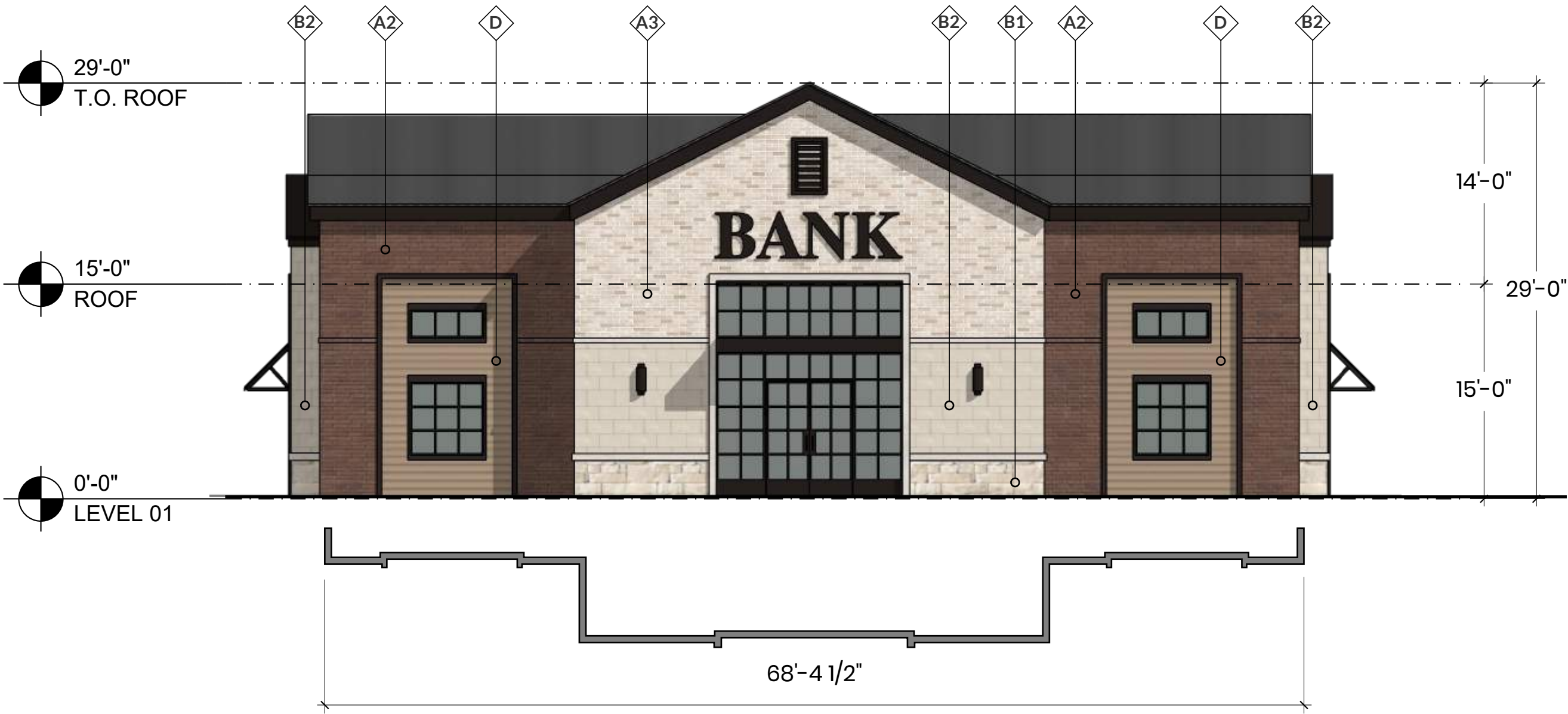
3 FRONT ELEVATION - BANK SCALE: 1/8" = 1'-0"
