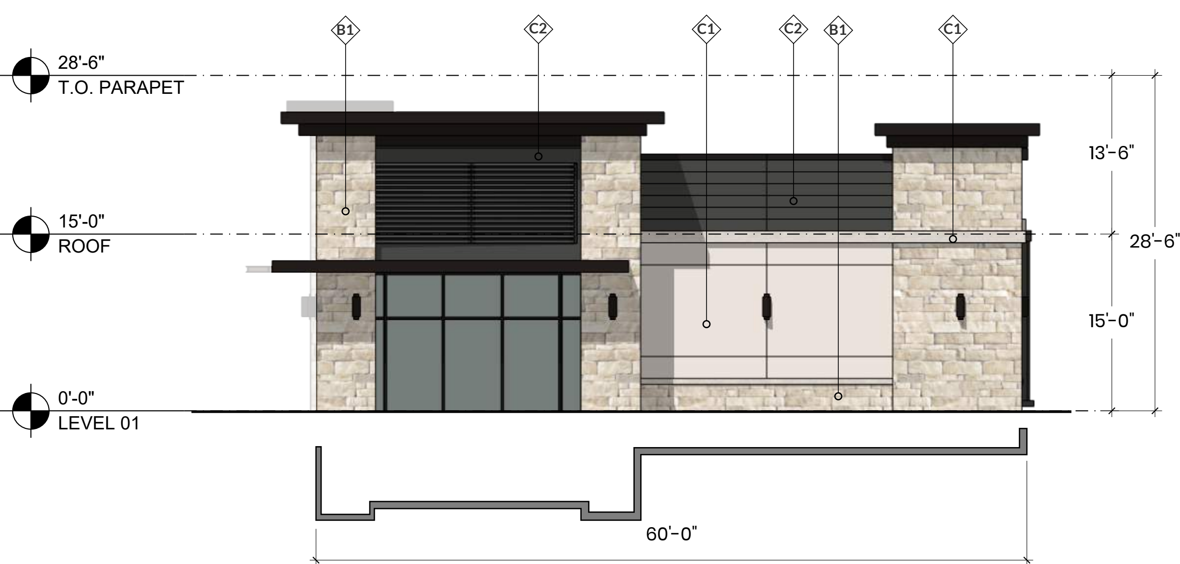
4 RIGHT ELEVATION - IN-LINE RETAIL SCALE: 1/8" = 1'-0"
