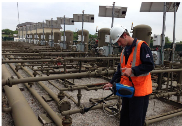
Example of infrared methane monitoring after a leak has been identified with the OGI equipment.
