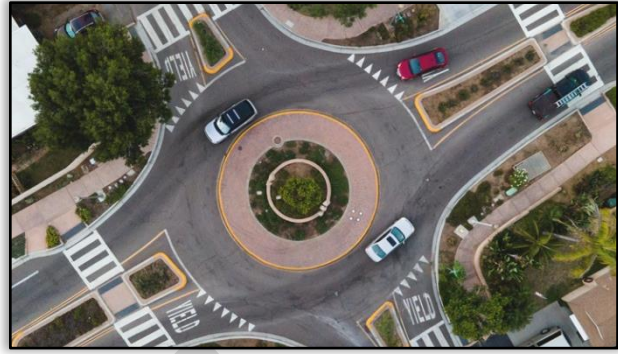
Figure 4. Typical Crosswalk Layout at a Roundabout Source: How to Drive in a Roundabout PEMCO Insurance
