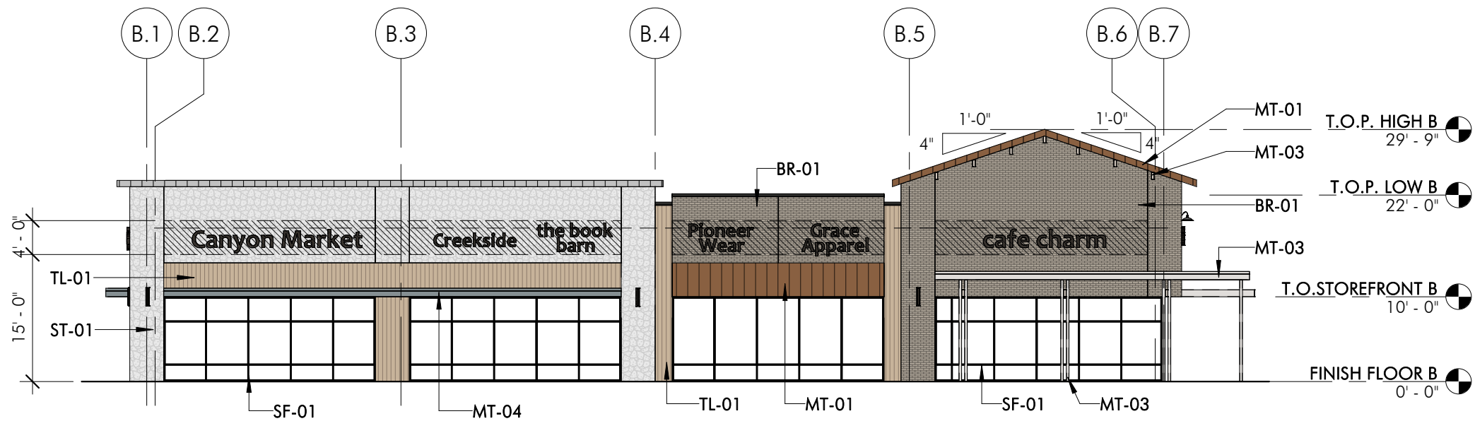
ZPD - BLDG B - NORTH ELEVATION|2 1/16" = 1'-0"
