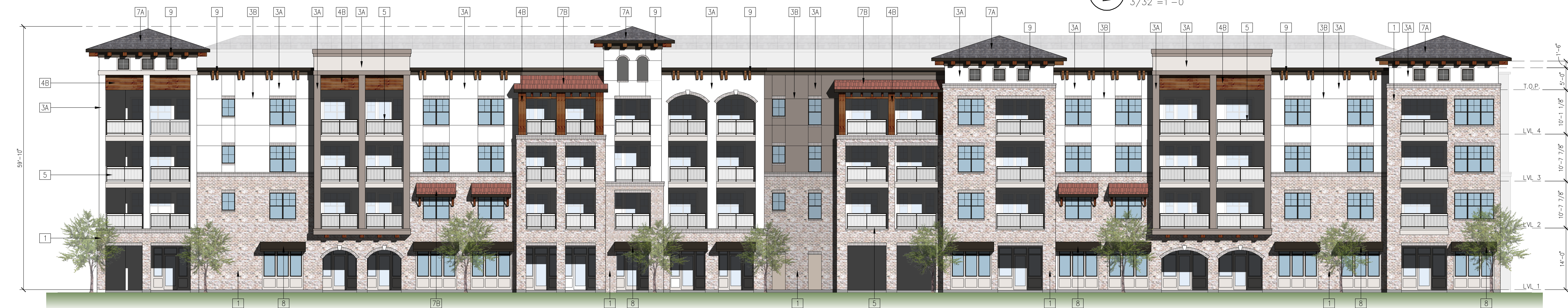
1 BLDG TYPE 1 - FRONT ELEVATION 3/32"=1'-0"
