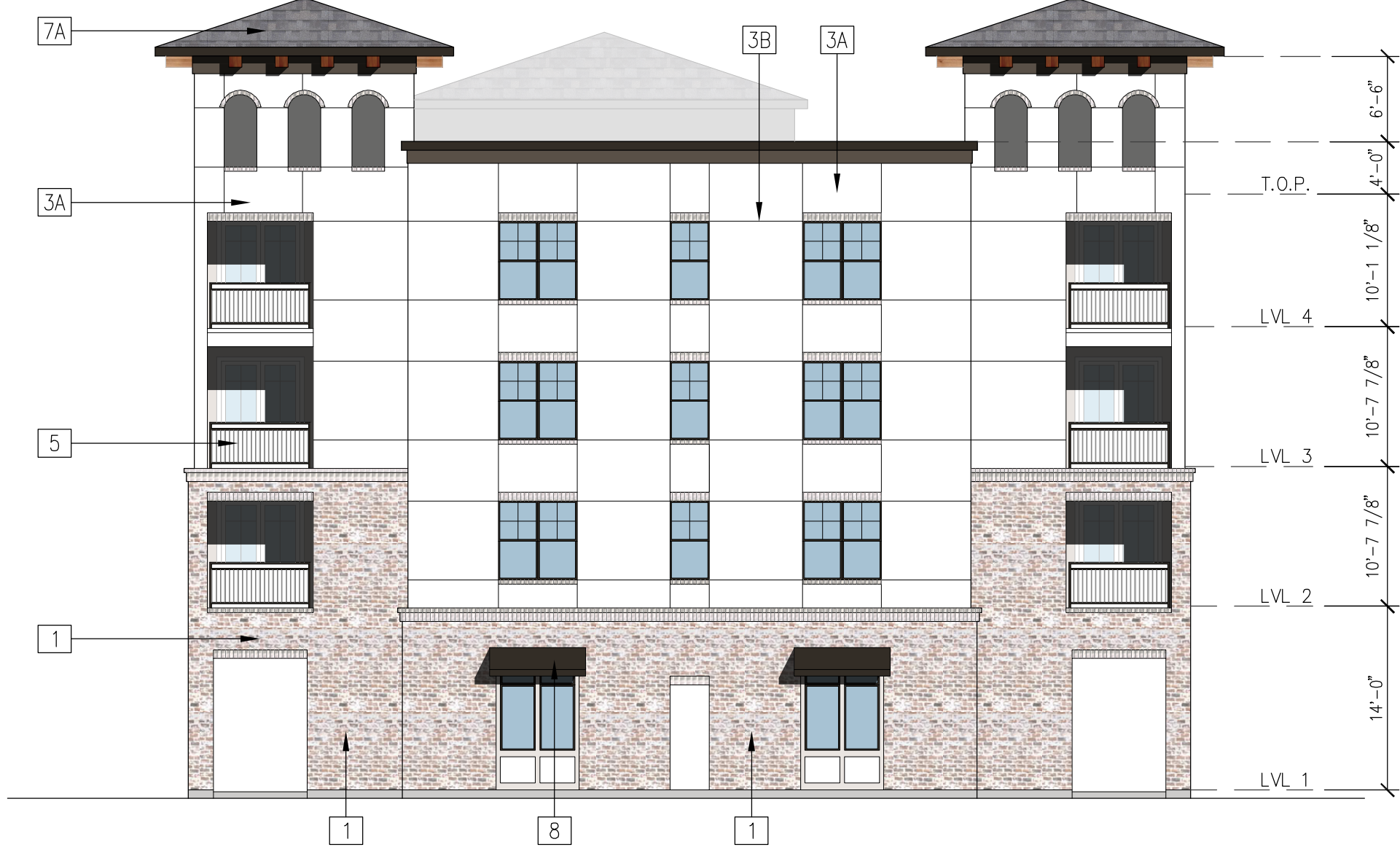
4 BLDG TYPE 2 - LEFT ELEVATION 3/32"=1'-0"
