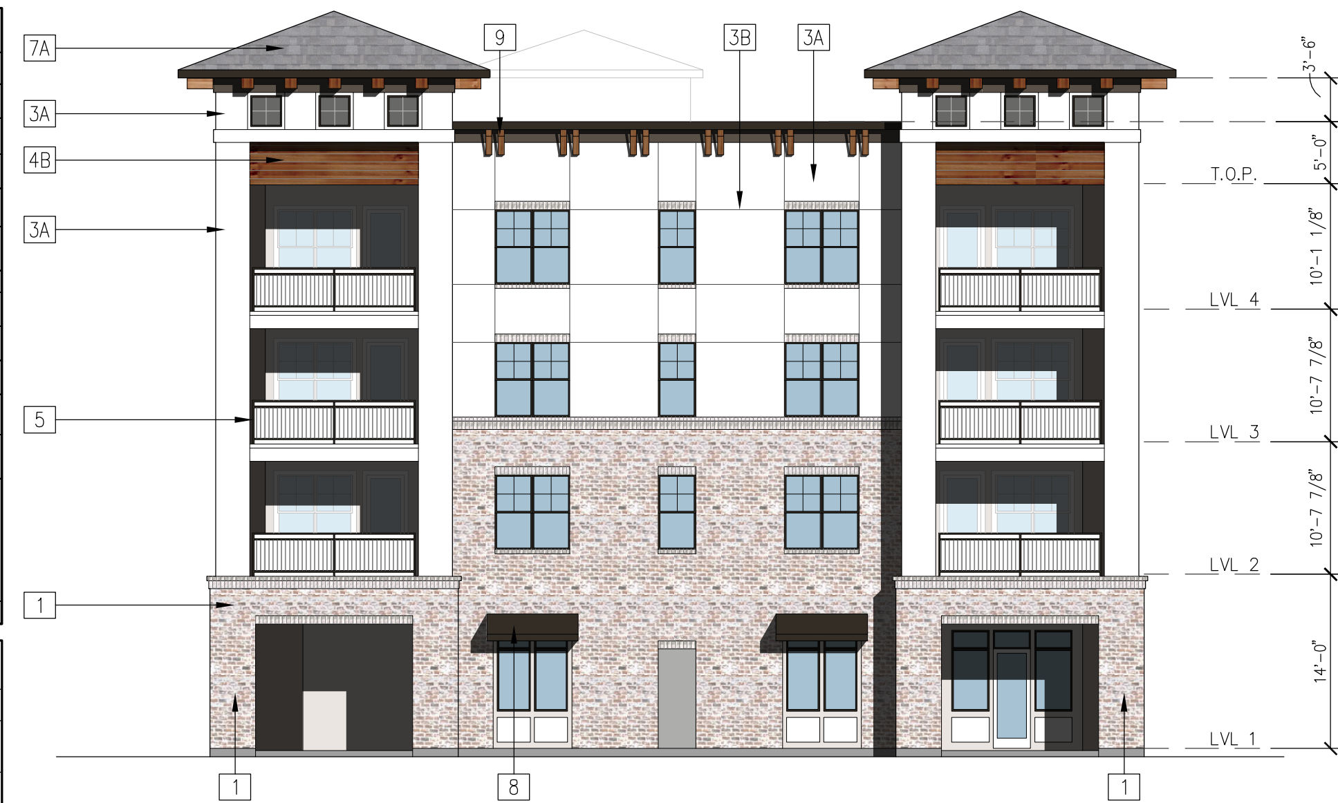
4 BLDG TYPE 1 - LEFT ELEVATION 3/32"=1'-0"
