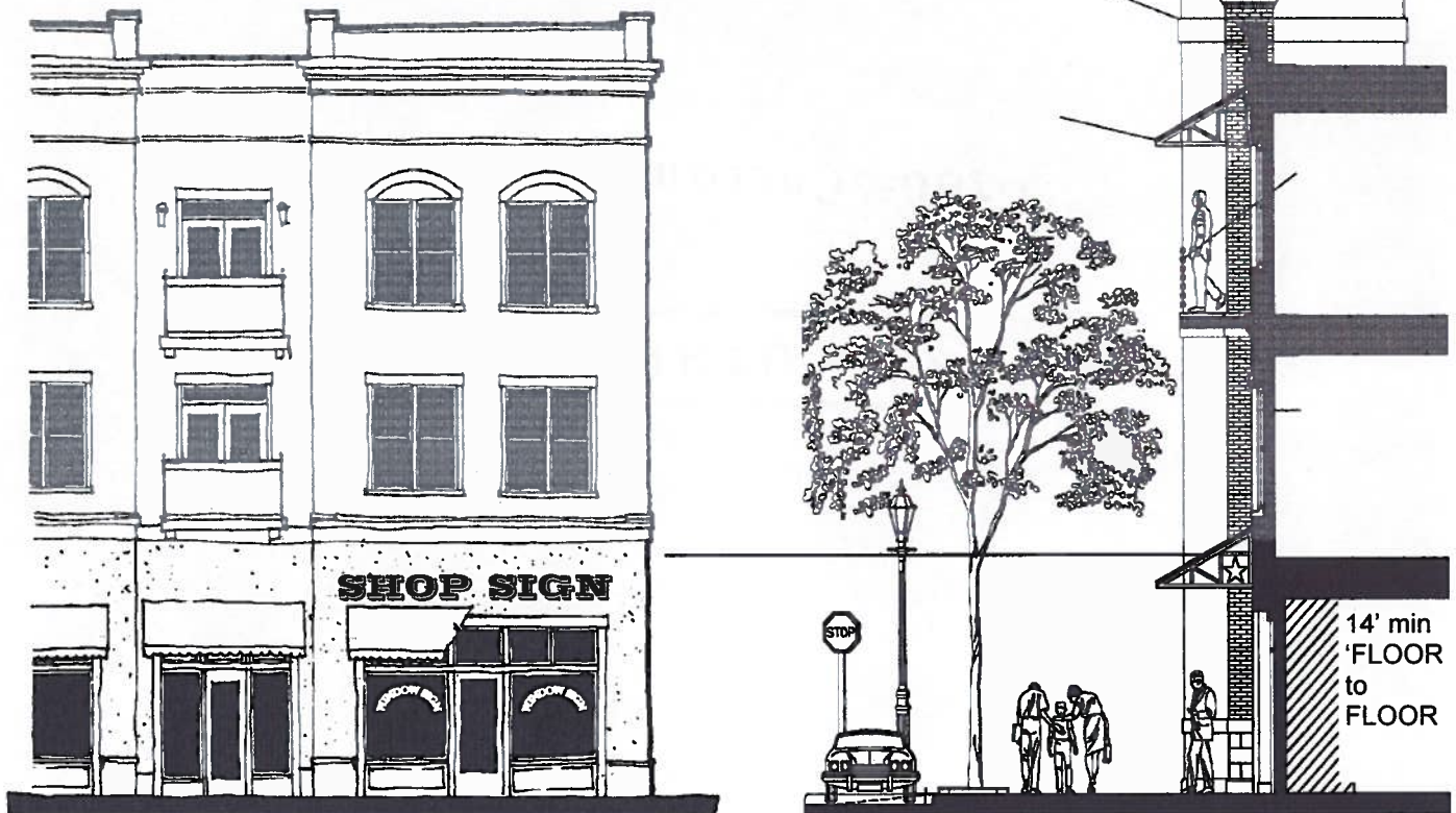
Figure 7.2: Ground floor built to commercial standards
