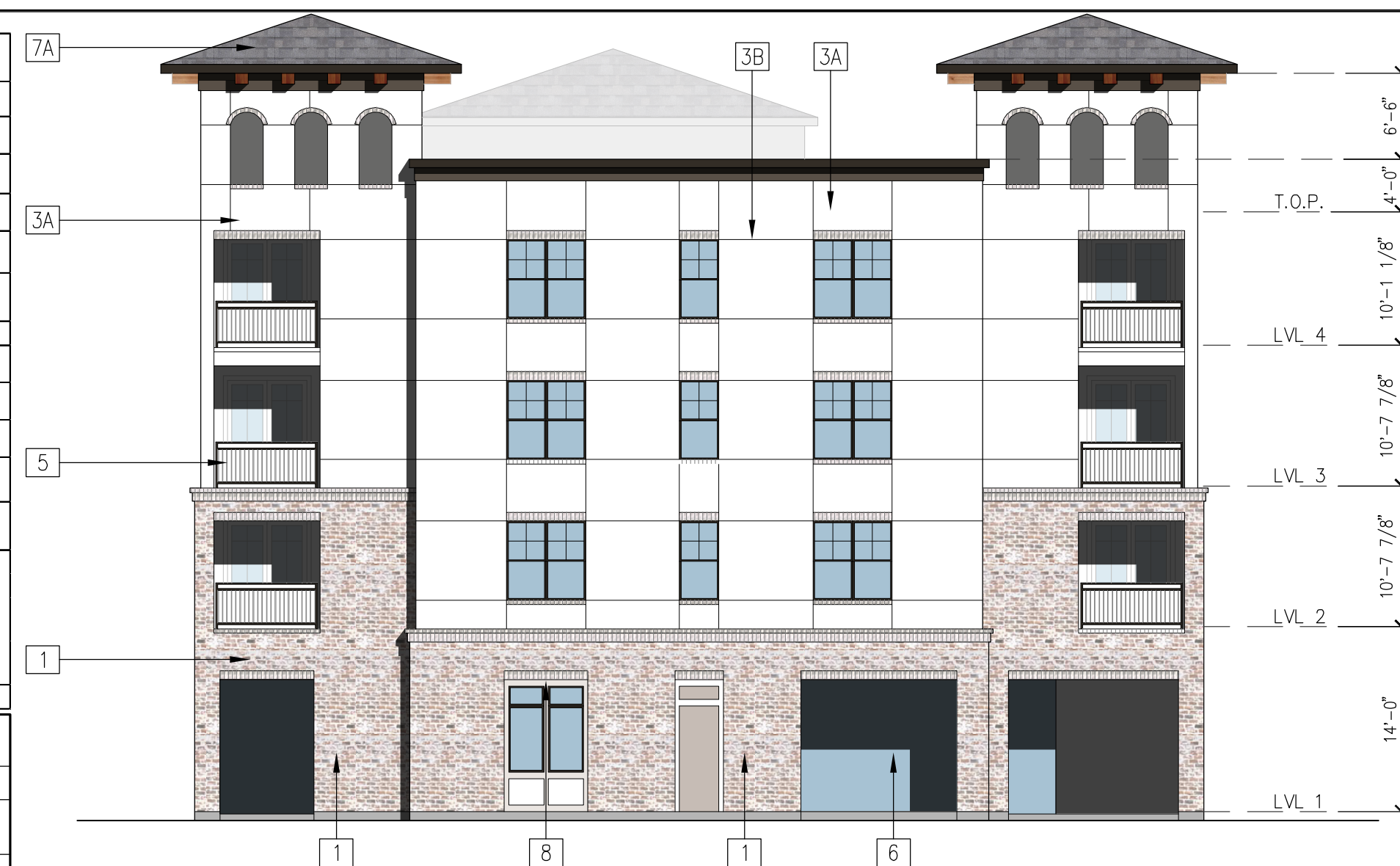
4 BLDG TYPE 2A - LEFT ELEVATION 3/32"=1'-0"
