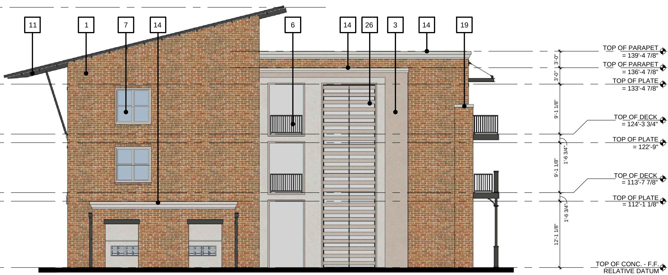
02 INTERIOR LOT SIDE ELEVATION (SOUTH) SCALE: 3/32" = 1'-0" BLDG #7
