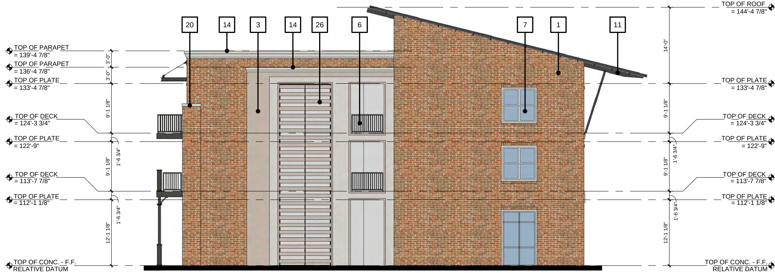
03 INTERIOR LOT SIDE ELEVATION (NORTH) SCALE: 3/32" = 1'-0" BLDG #7
