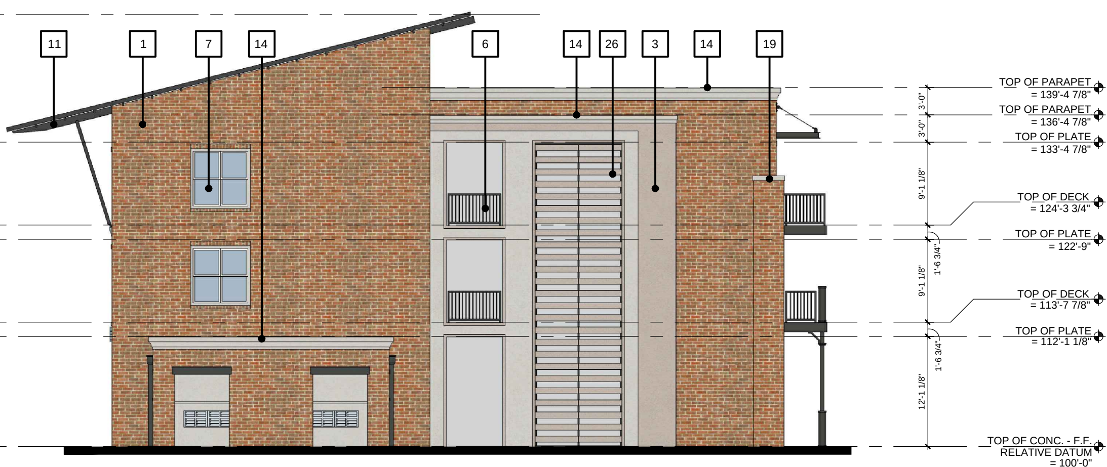
02 INTERIOR LOT SIDE ELEVATION (SOUTH) SCALE: 3/32" = 1'-0" BLDG #7
