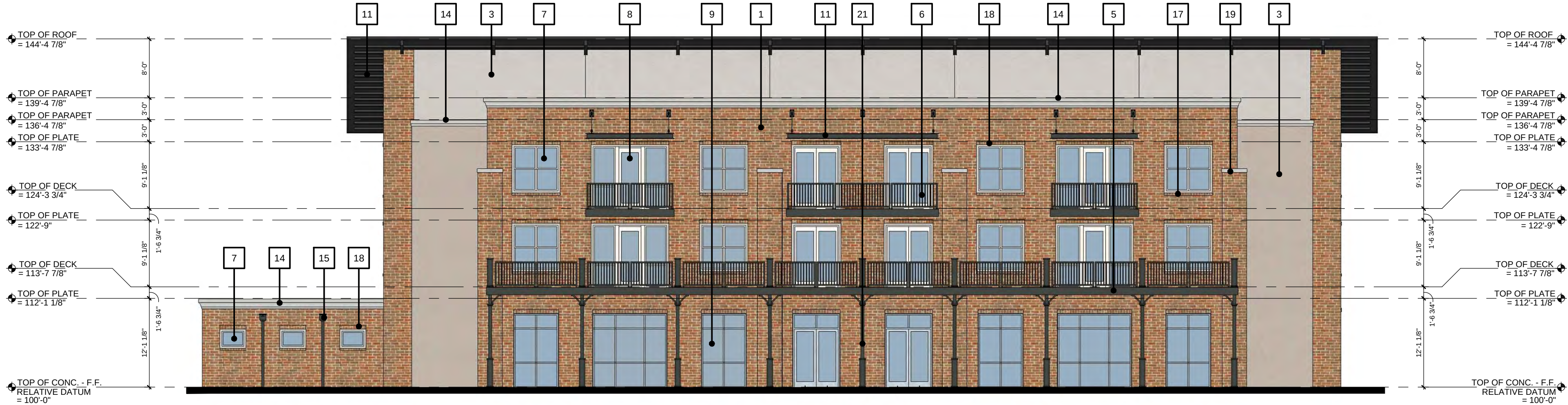
04 INTERIOR LOT POOL ELEVATION (EAST) SCALE: 3/32" = 1'-0" BLDG #7
