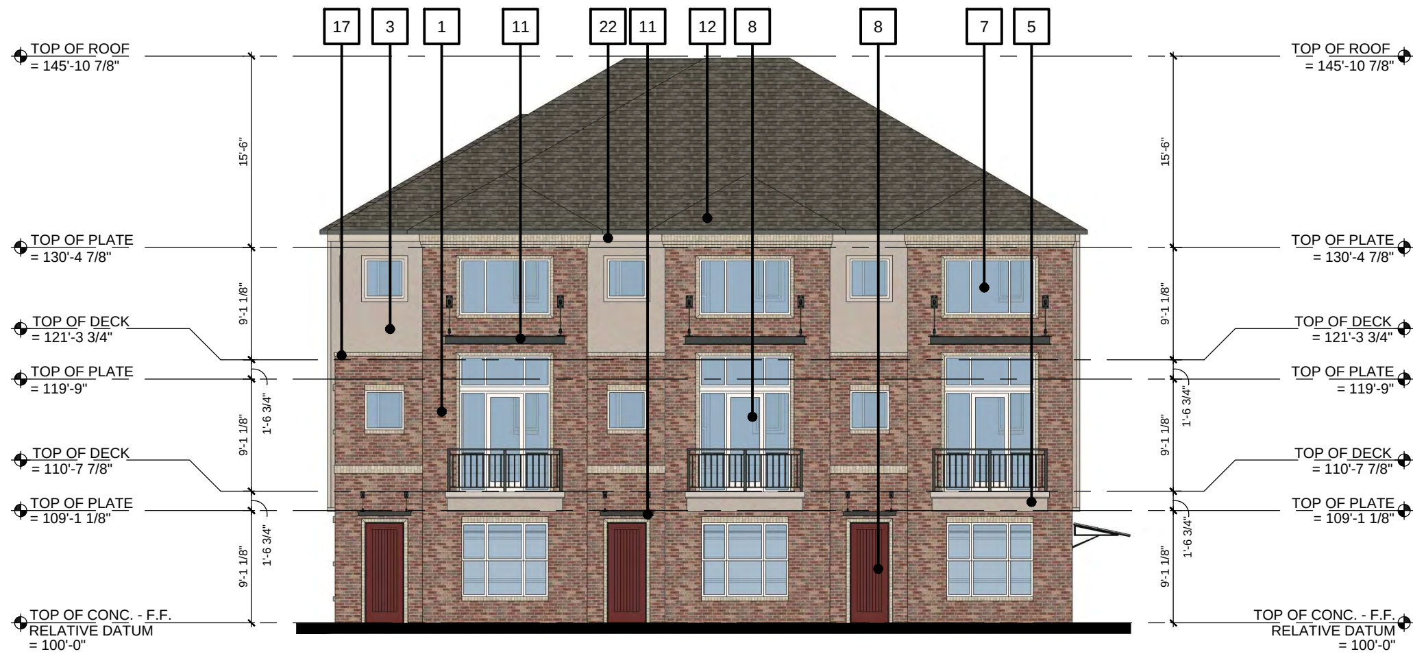
01 1ST AVENUE ELEVATION (NORTH) SCALE: 3/32" = 1'-0" BLDG #6
