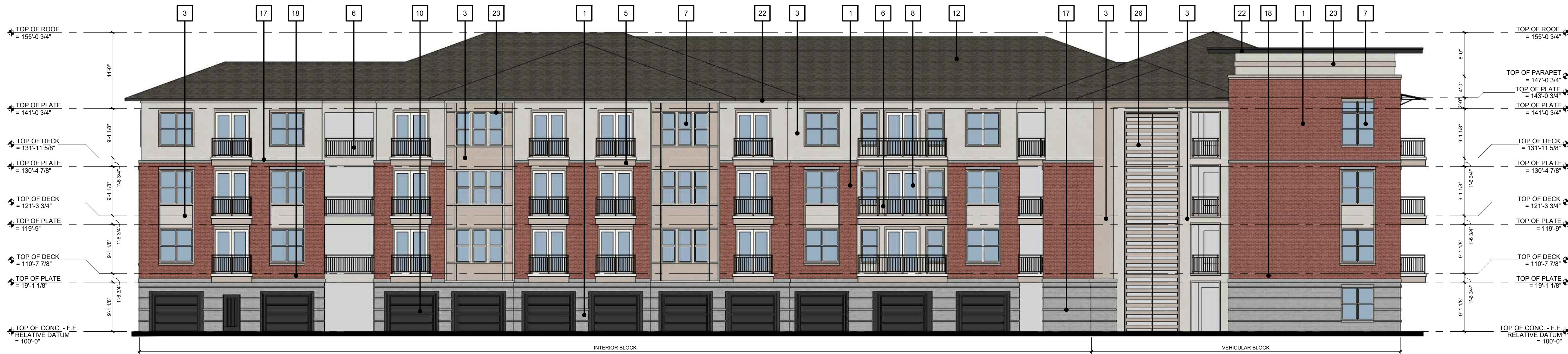
01 SIDE / INTERIOR LOT ELEVATION (SOUTH) SCALE: 3/32" = 1'-0" BLDG #5
