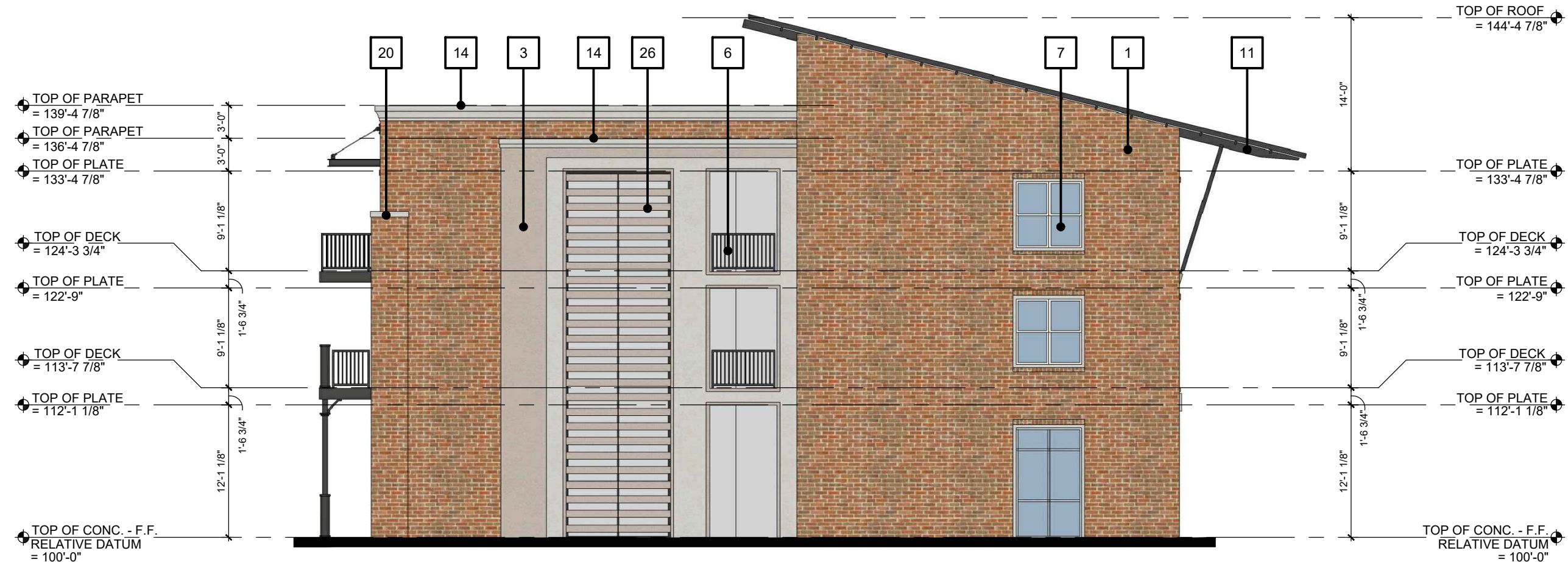
03 INTERIOR LOT SIDE ELEVATION (NORTH) SCALE: 3/32" = 1'-0" BLDG #7
