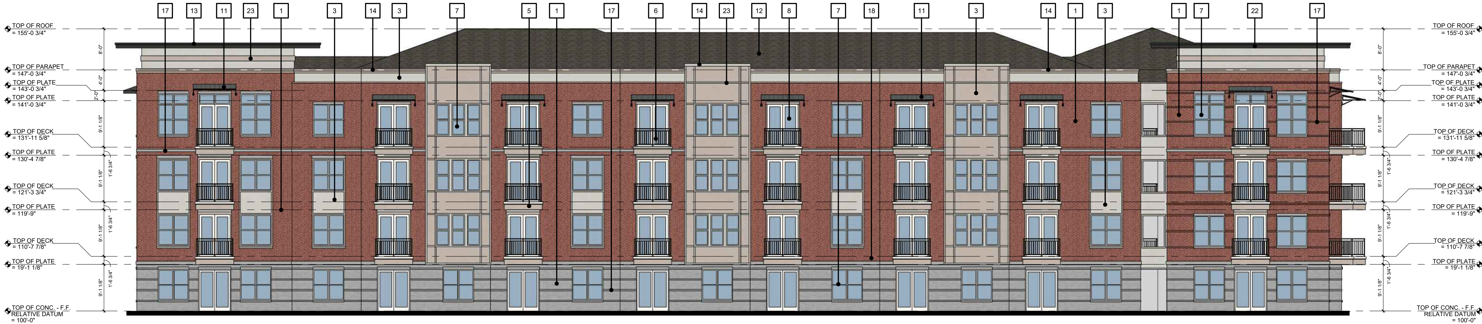
01 COMMUNITY DRIVE ELEVATION (SOUTH) SCALE: 3/32" = 1'-0" BLDG #4
