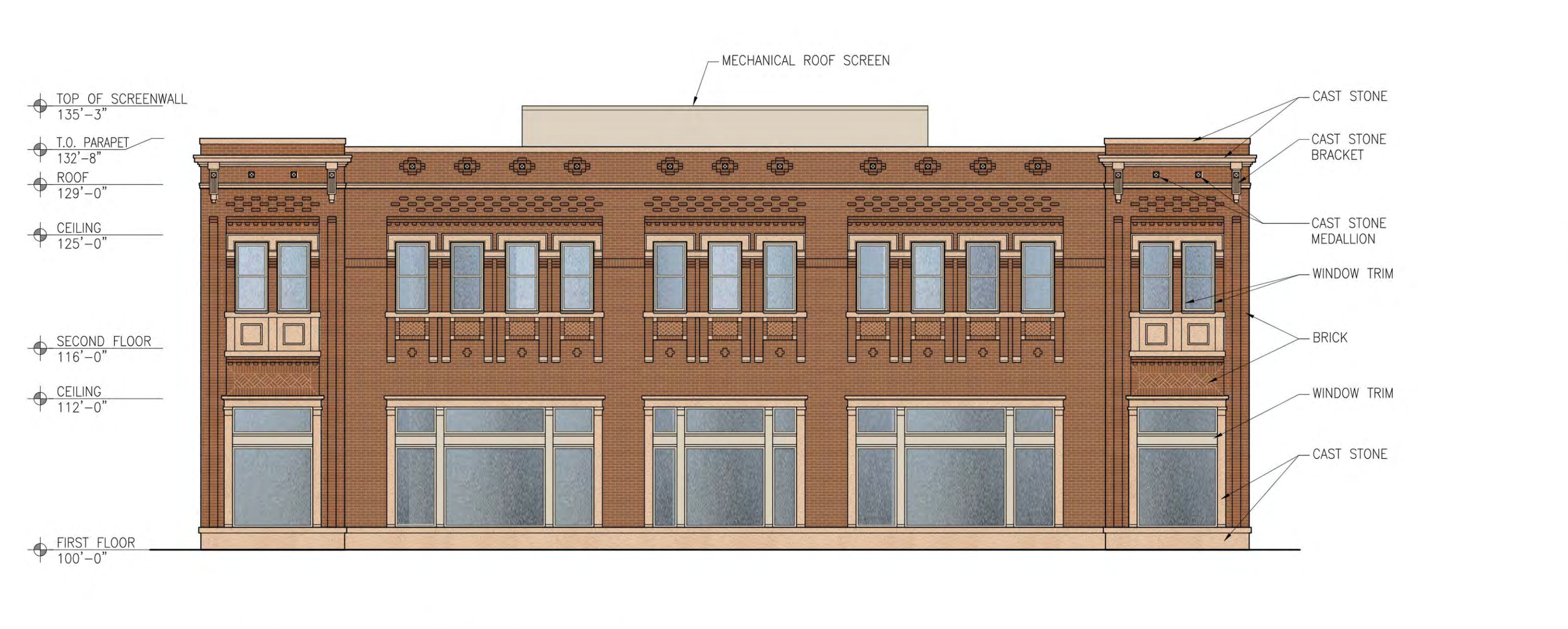
04 EXTERIOR ELEVATION - NORTHEAST SCALE: 1/8"=1'-0"
