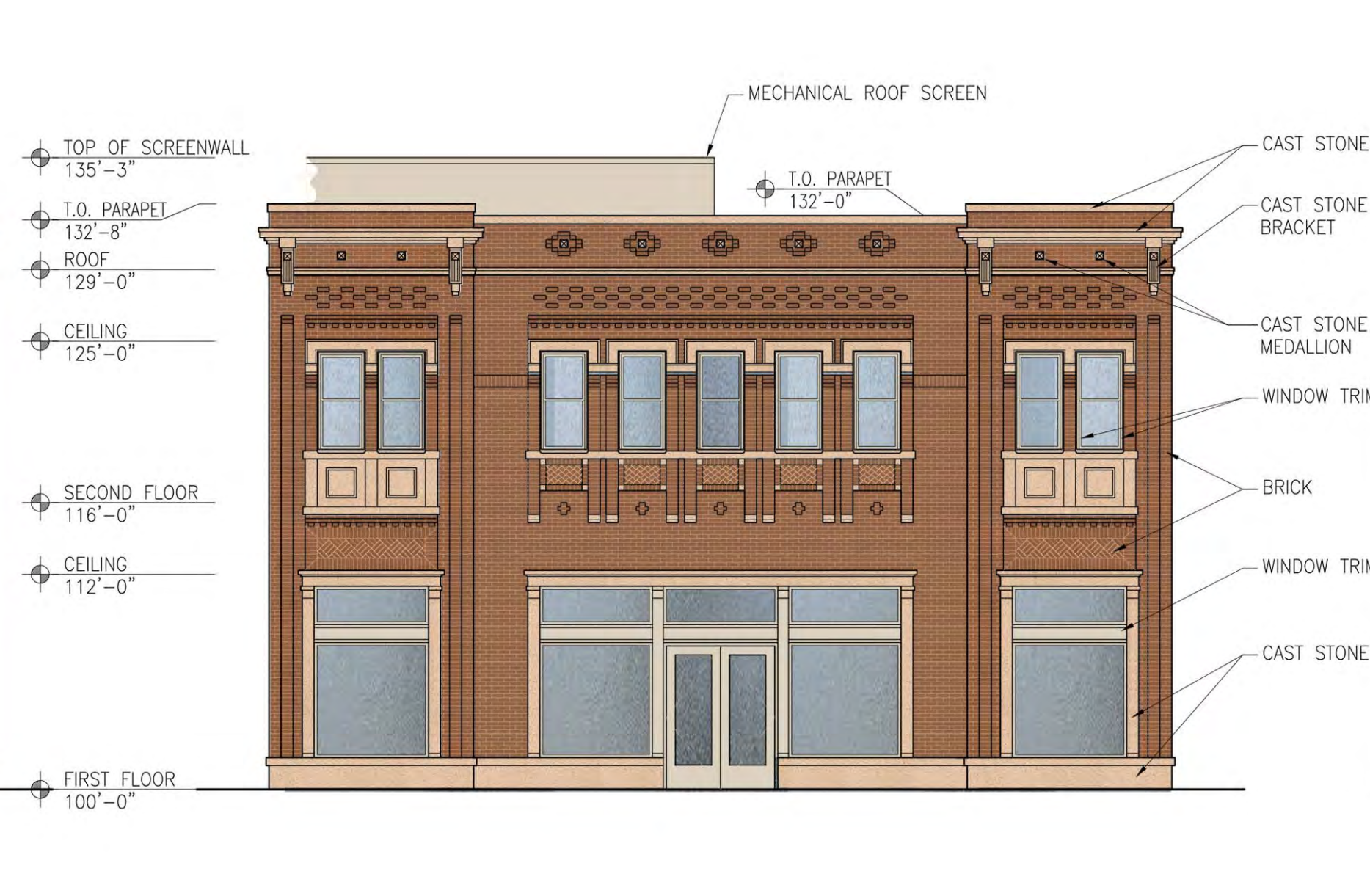
05 EXTERIOR ELEVATION - NORTH SCALE: 1/8"=1'-0"
