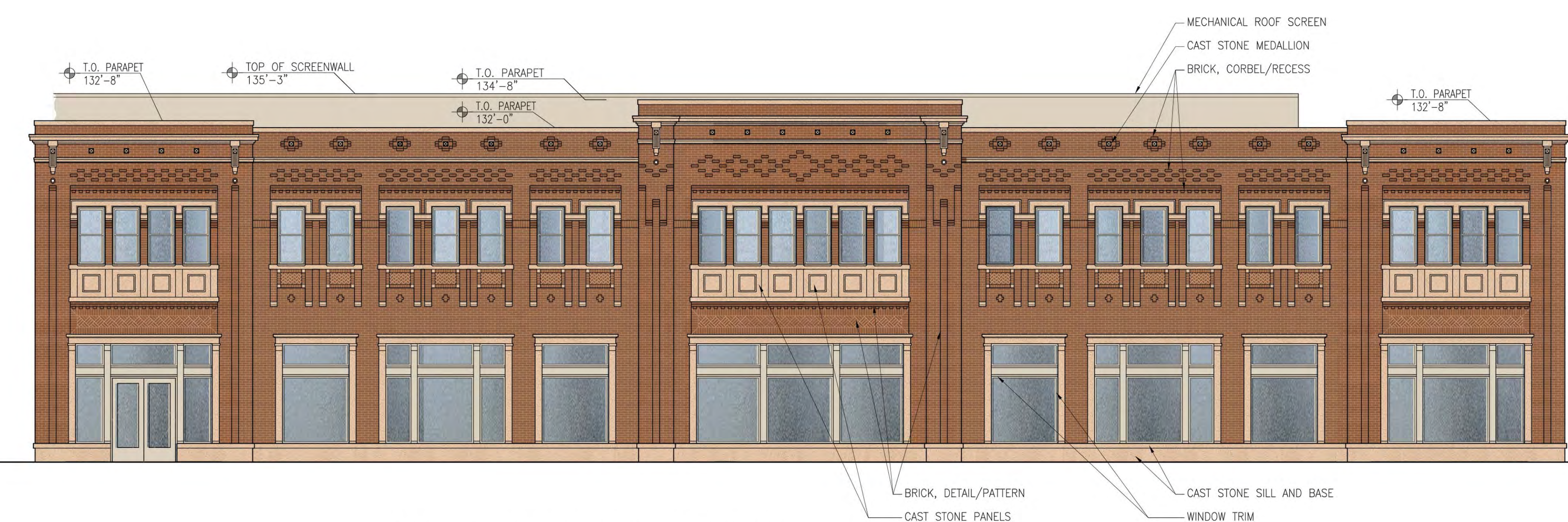
02 EXTERIOR ELEVATION - SOUTHEAST SCALE: 1/8"=1'-0"
