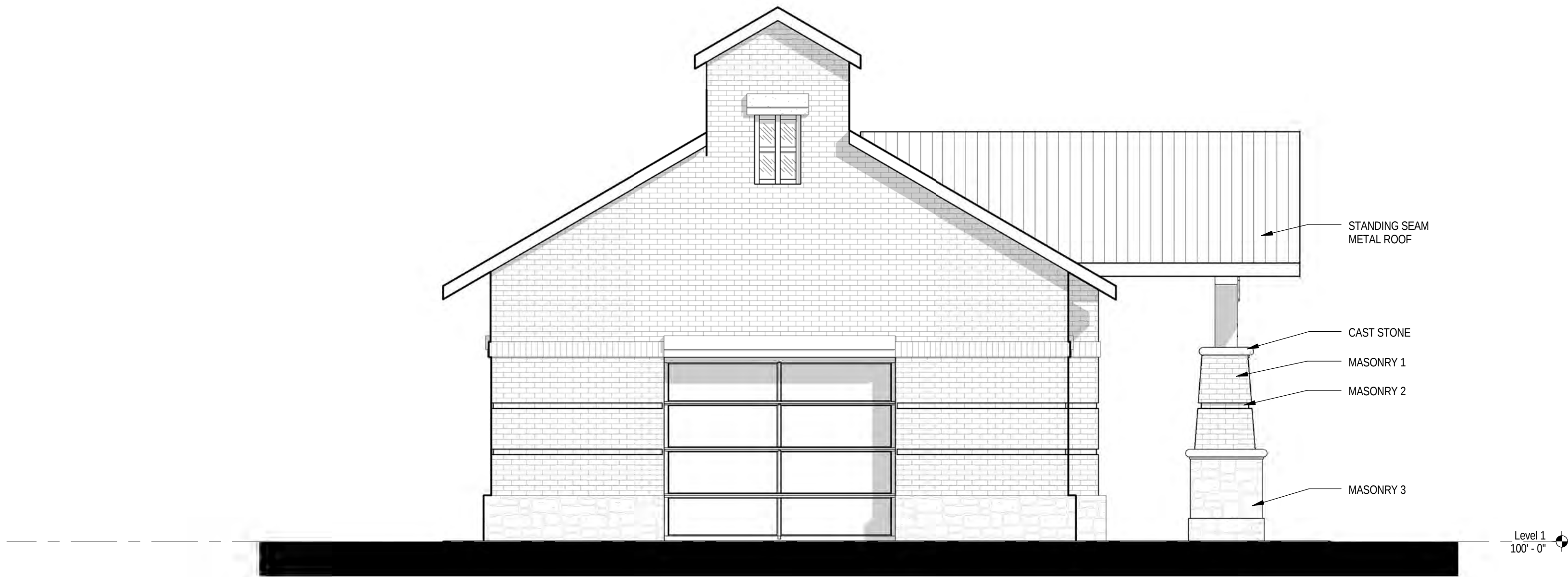
2 Building 2 West Elevation 1/4" = 1'-0"
