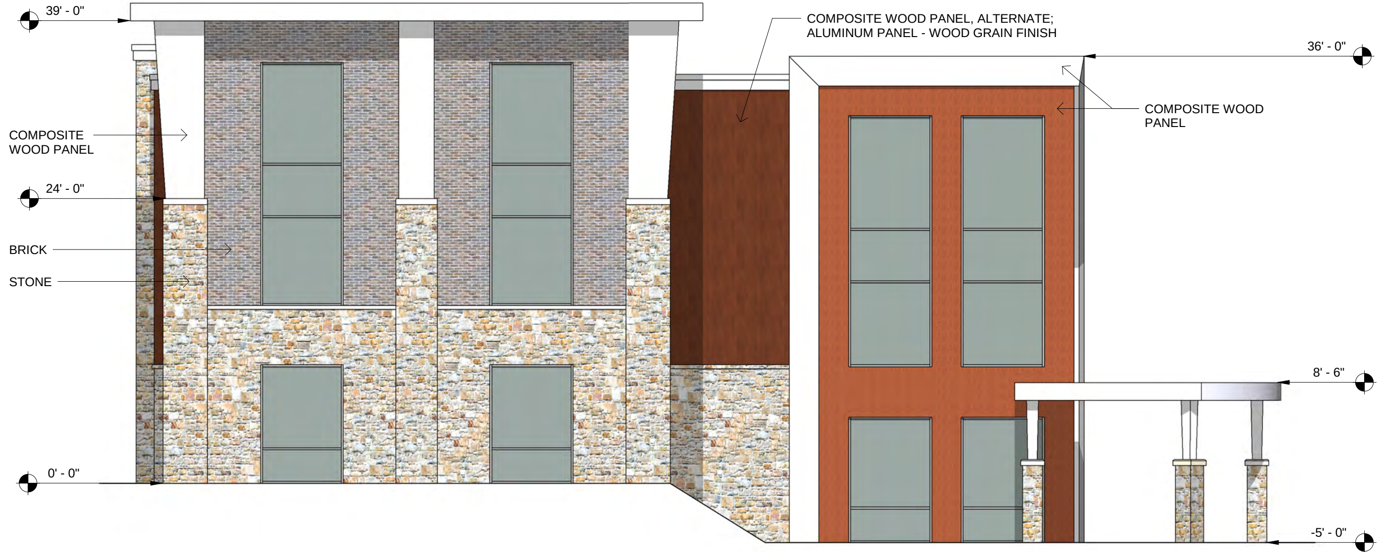
② BUILDING 6 - ELEVATION - NORTH 1/8" = 1'-0"
